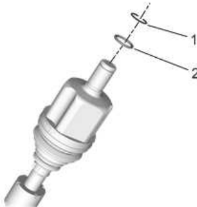
Fig. 9: Front Wheel Drive Shaft Retaining Ring And Seal
