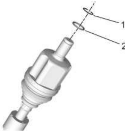
Fig. 8: Front Wheel Drive Shaft Retaining Ring And Seal
