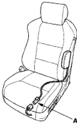
Fig. 30: Identifying Airbag 2P Connectors And Floor Wire Harness Courtesy of AMERICAN HONDA MOTOR CO., INC.
