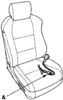
Fig. 163: Identifying Front Passenger's Seat Belt Buckle Switch 3P Connector (A) Courtesy of AMERICAN HONDA MOTOR CO., INC.
