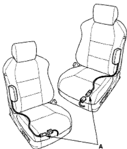
Fig. 203: Identifying Side Airbag Harness 2P Connector (A) Courtesy of AMERICAN HONDA MOTOR CO., INC.
