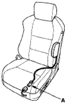
Fig. 212: Identifying Side Airbag 2P Connector And Floor Wire Harness Courtesy of AMERICAN HONDA MOTOR CO., INC.
