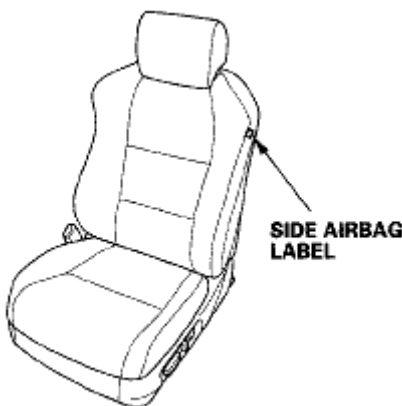
Fig. 26: Identifying Seat Side Airbag Label
