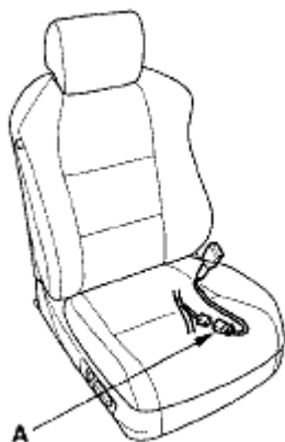
Fig. 160: Identifying Front Passenger's Seat Wire Harness 3P Connector And Front Passenger's Seat Belt Buckle Switch 3P Connector (A)
