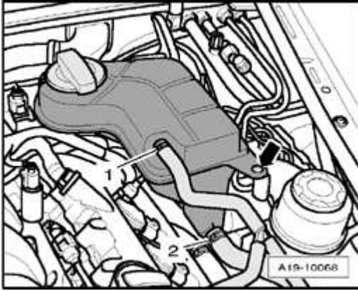
Fig. 132: Removing Coolant Hoses At Coolant Expansion Tank Courtesy of VOLKSWAGEN UNITED STATES, INC.
