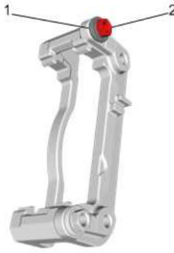
Fig. 12: Upper Guide Pin Seal And Guide Pin Seal Courtesy of GENERAL MOTORS COMPANY
