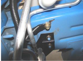
G102 (at right front longitudinal beam)
