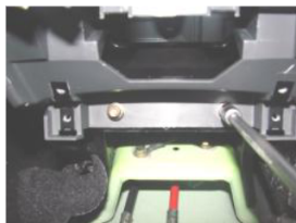
G207, 208(at secondary instrument panel)
