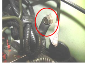
G101 (at left front longitudinal beam)
