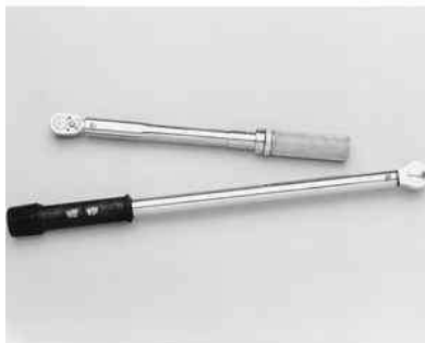
Fig. 6: Many repairs will require the use of a torque wrench to assure the components are properly fastened
