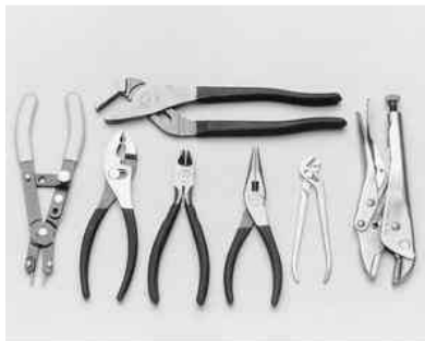
Fig. 4: An assortment of pliers, grippers and cutters will be handy for old rusted parts and stripped bolt heads
