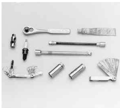
Fig. 10: A variety of tools and gauges should be used for spark plug gapping and installation
