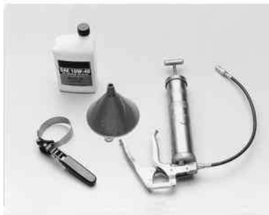
Fig. 8: A few inexpensive lubrication tools will make maintenance easier
