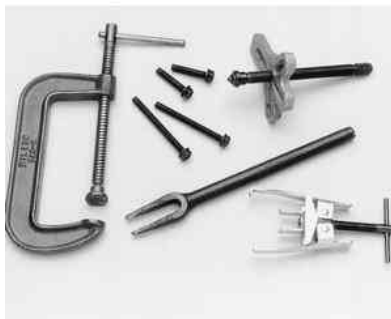
Fig. 9: Various pullers, clamps and separator tools are needed for many larger, more complicated repairs
