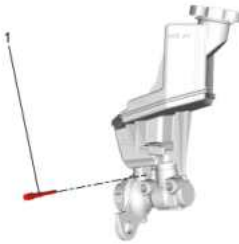
Fig. 13: Brake Master Cylinder Reservoir Bolt Courtesy of GENERAL MOTORS COMPANY
