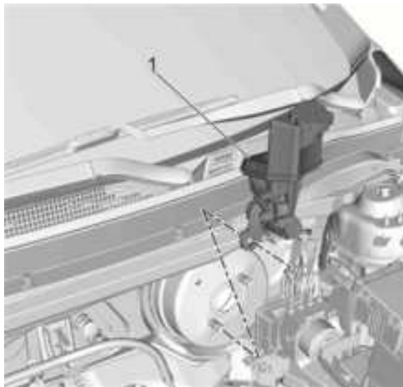
Fig. 131: Brake Master Cylinder Assembly Courtesy of GENERAL MOTORS COMPANY
