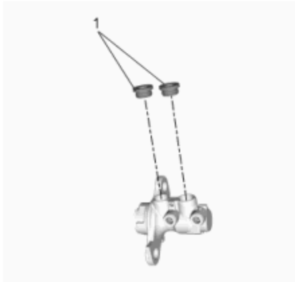
Fig. 11: Master Cylinder Reservoir Seals Courtesy of GENERAL MOTORS COMPANY
