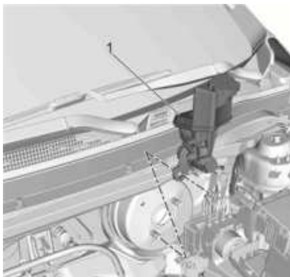
Fig. 19: Brake Master Cylinder Assembly Courtesy of GENERAL MOTORS COMPANY
