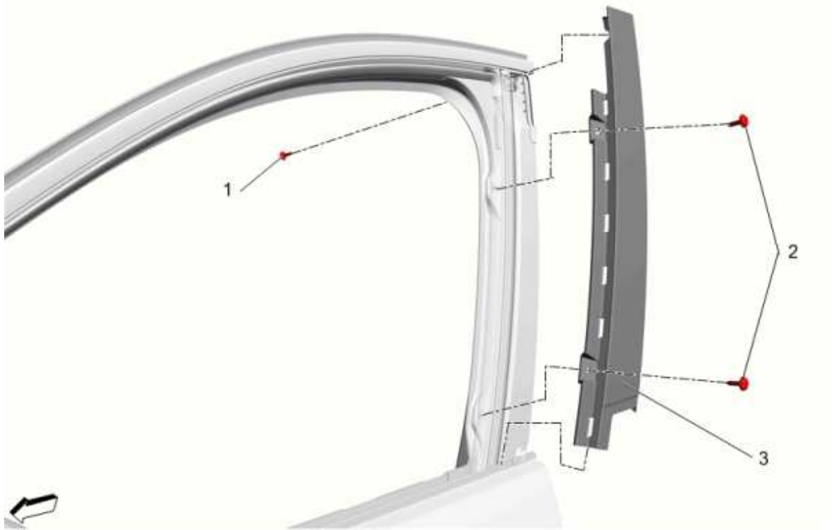
Fig. 48: Front Side Door Window Frame Rear Applique And Screws
