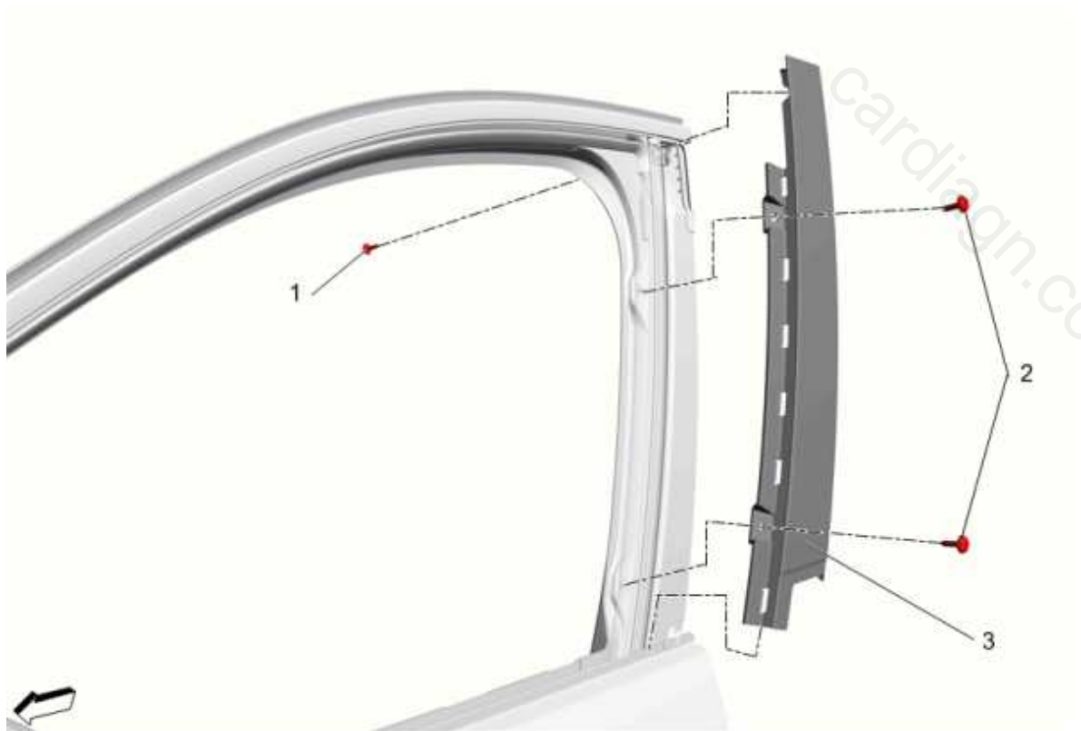
Fig. 77: Front Side Door Window Frame Rear Applique And Screws
