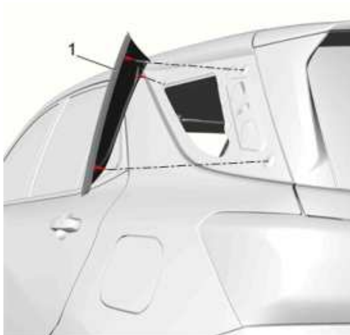
Fig. 119: Placing Window Courtesy of GENERAL MOTORS COMPANY
