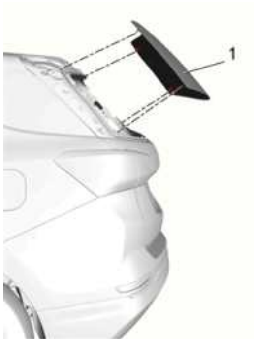
Fig. 127: Placing Window Courtesy of GENERAL MOTORS COMPANY
