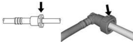
Fig. 36: Variants Of Sliding Retainer Style Connectors Courtesy of GENERAL MOTORS COMPANY
