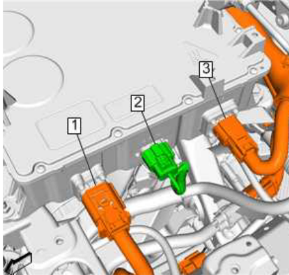
Fig. 38: Drive Motor Battery Charger Electrical Connector
