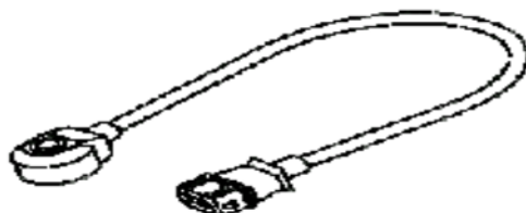
Chart 3-4 Exterior drawing of knock sensor
