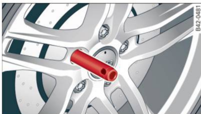
Fig. 161 Wheel change: alignment pin inside the top hole
