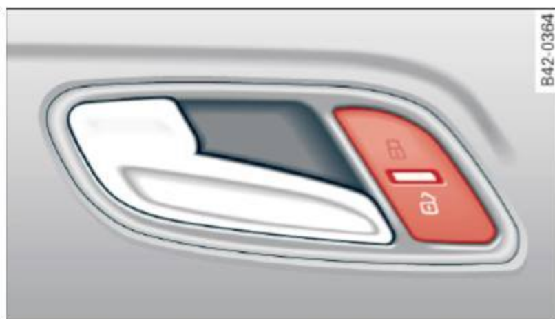
Fig. 34 Section from driver's door: Power locking switch
