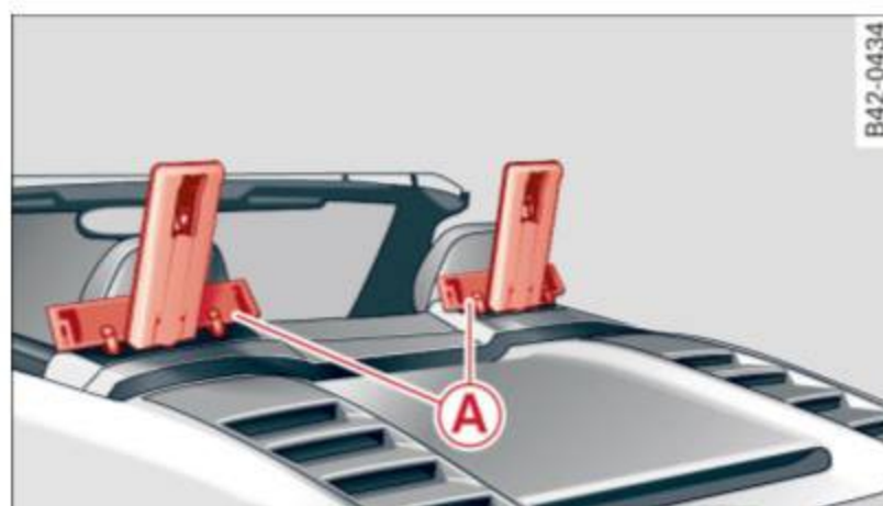
Fig. 111 Deployed rollbar with convertible top frame facing upward
