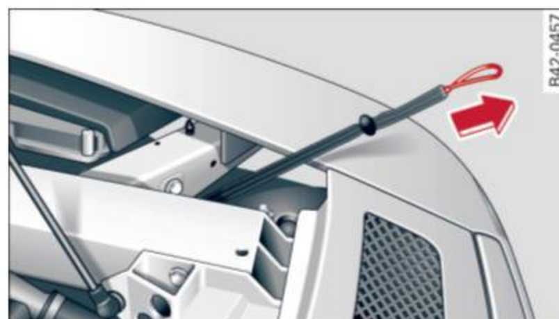
Fig. 138 Engine compartment: releasing the fuel filler flap using the emergency release
