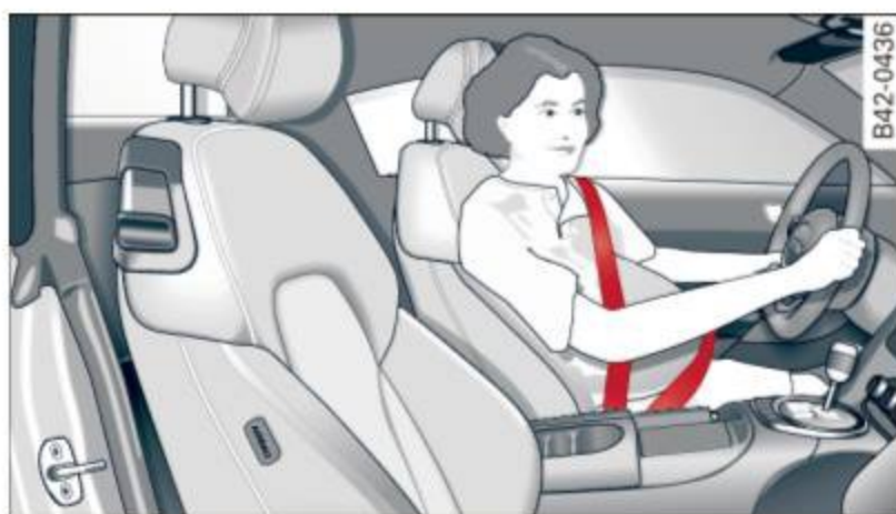
Fig. 120 Safety belt position during pregnancy
