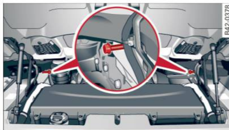
Fig. 50 Engine compartment: installing the emergency operation bolts
