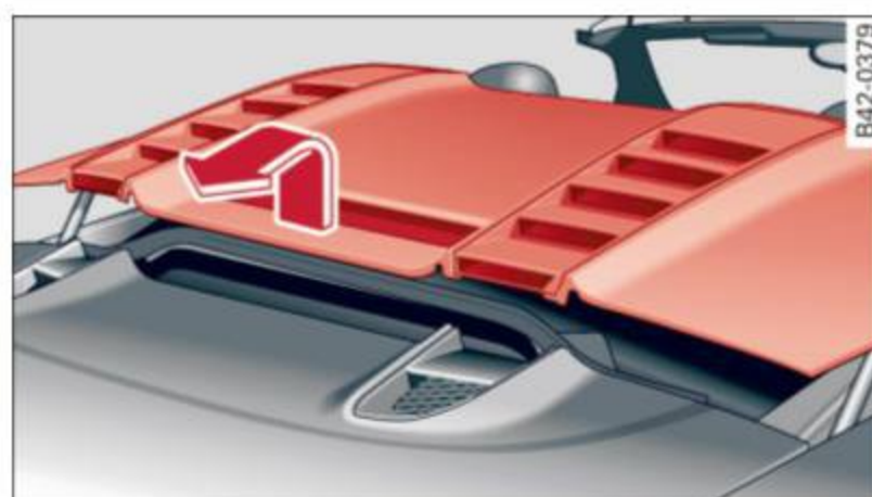
Fig. 51 Raising the storage bay lid and pulling it back
