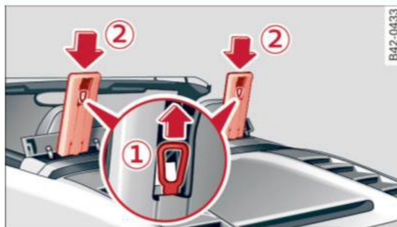
Fig. 110 Deployed rollbar with release loop
