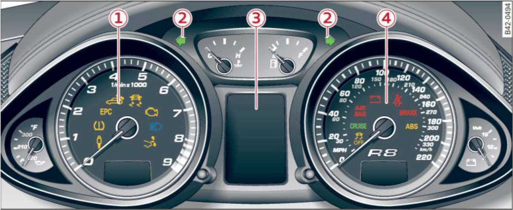
Fig. 6 Instrument cluster with warning/indicator lights
