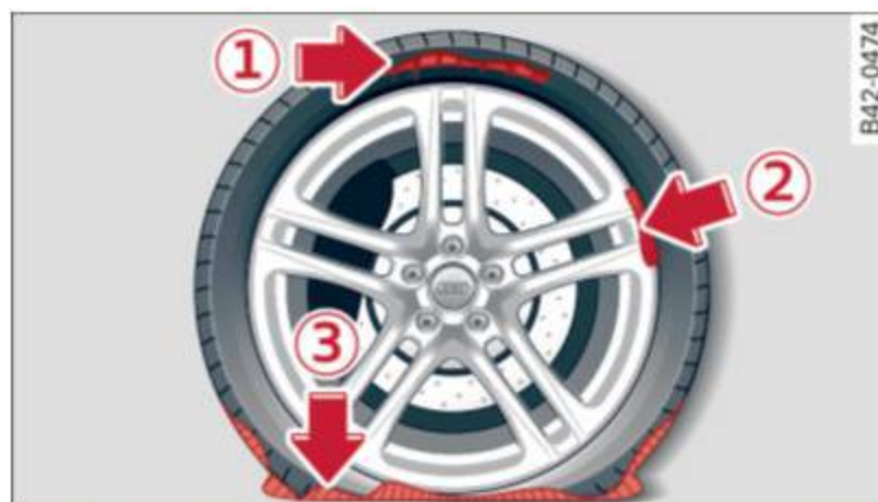
Fig. 155 Tire damage for which the Tire Mobility System is not suited
