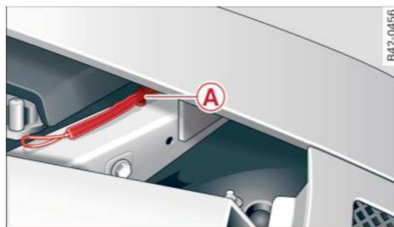
Fig. 137 Engine compartment: loosening the fuel filler flap cable
