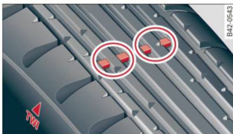
Fig. 152 Tire tread: tread wear indicators (TWI)
