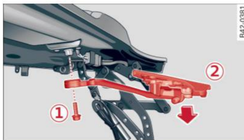
Fig. 53 Convertible top storage bay lid: removing the cover
