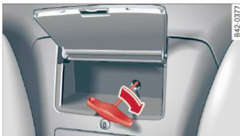
Fig. 49 Upper storage compartment: using the Allen wrench as a crank to lower the rear window
