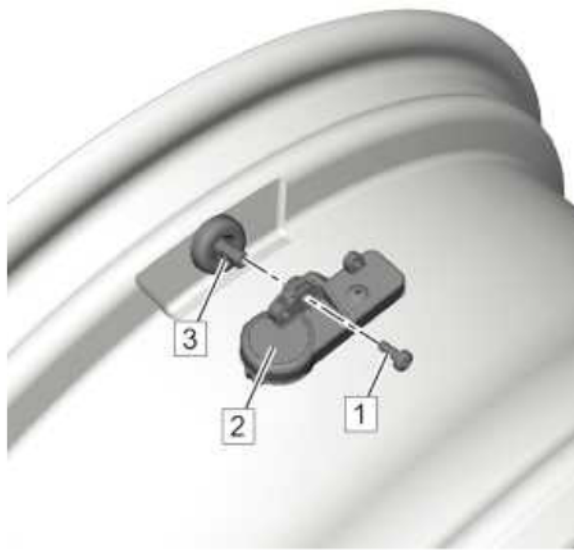
Fig. 1: Tire Pressure Transmitter And Valve Stem
