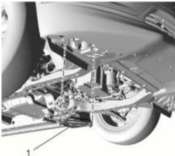
Fig. 23: Lower Deflector Panel Insert
