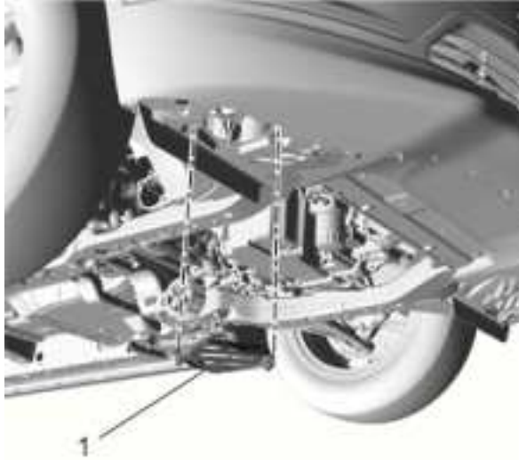
Fig. 22: Lower Deflector Panel Insert
