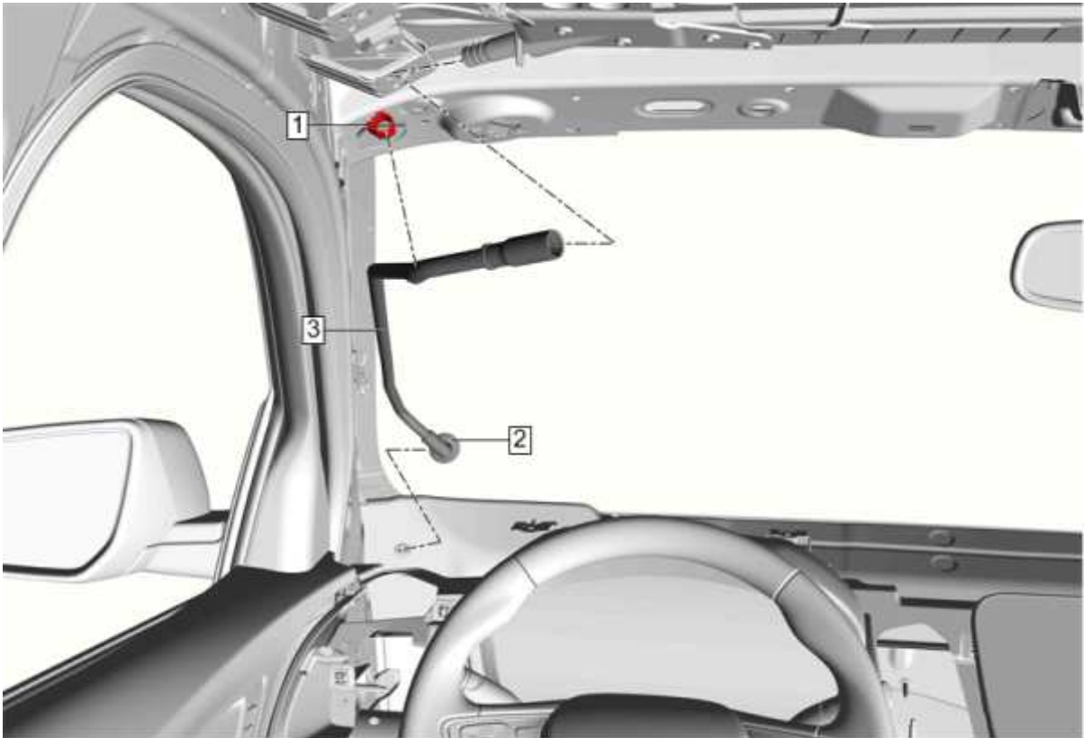
Fig. 7: Sunroof Housing Front Drain Hose (Terrain Left Side) Courtesy of GENERAL MOTORS COMPANY
