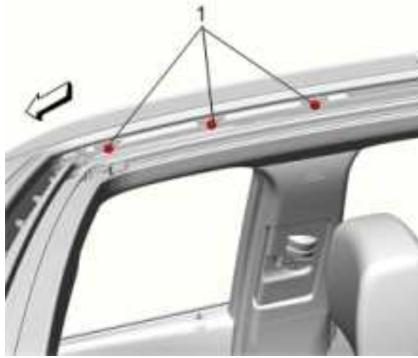
Fig. 42: Front Sunroof Window Rear Screws
