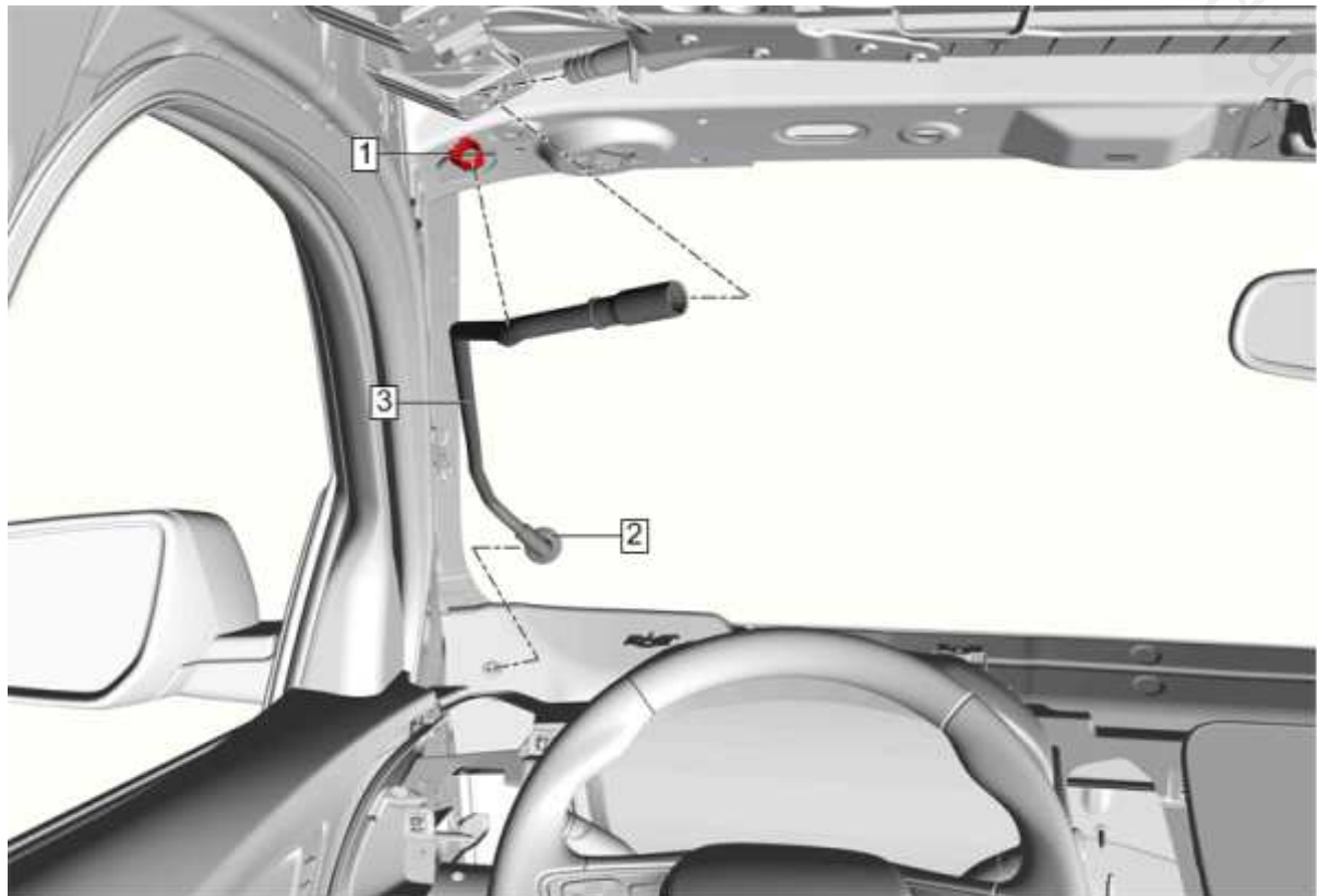
Fig. 5: Sunroof Housing Front Drain Hose (Equinox Left Side)
