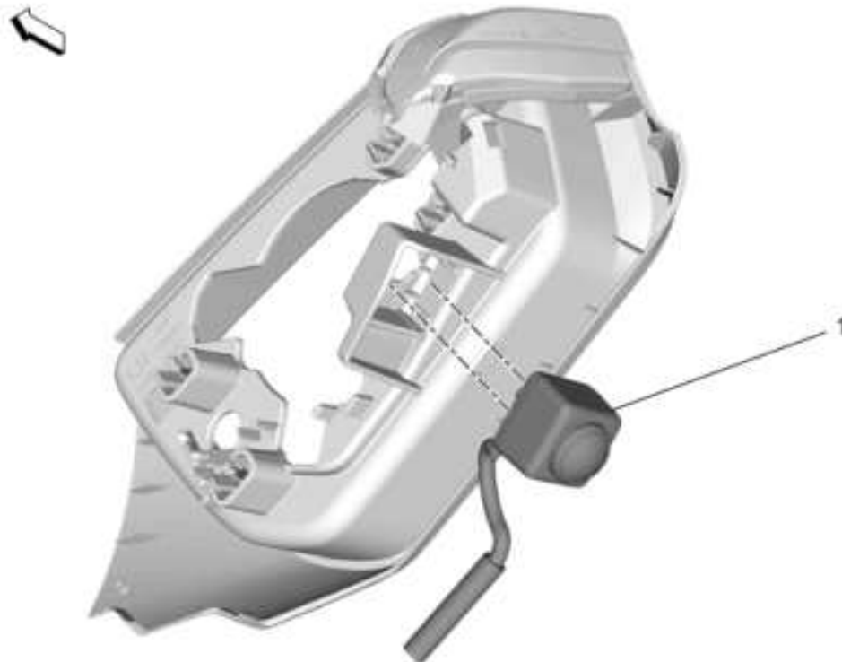
Fig. 12: Side View Driver Information Camera Courtesy of GENERAL MOTORS COMPANY
