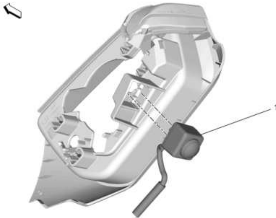
Fig. 11: Side View Driver Information Camera Courtesy of GENERAL MOTORS COMPANY
