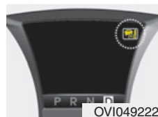
SCC malfunction indicator (if equipped)
