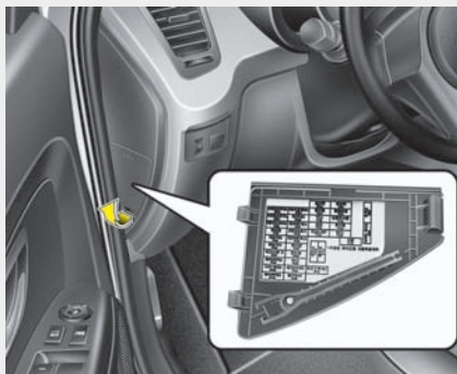
Inner fuse panel
