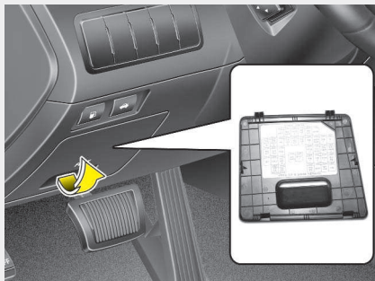
Instrument panel fuse panel
