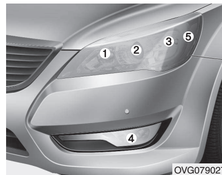
Headlight, position light, turn signal light, front fog light bulb replacement
