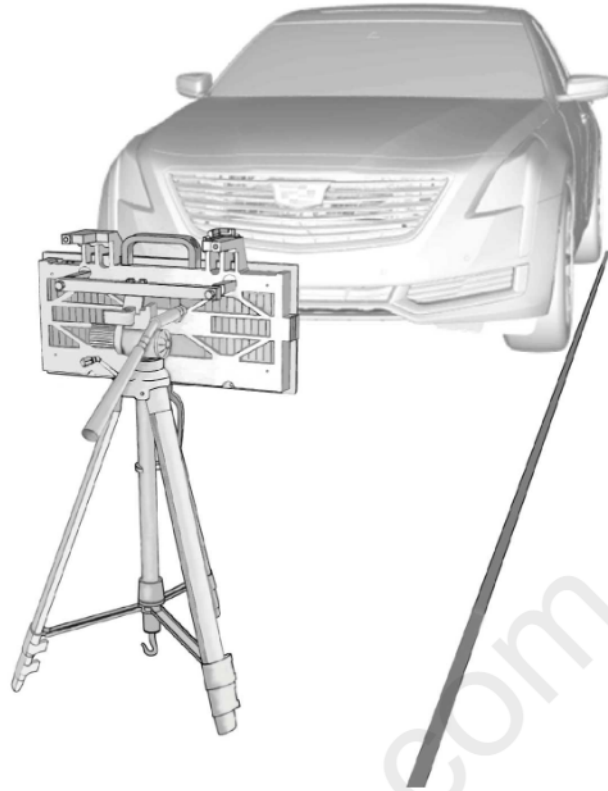
Fig. 28: View Of Night Vision Camera Alignment Procedure
