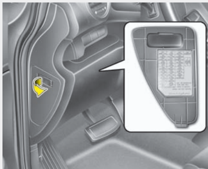
Inner fuse panel
