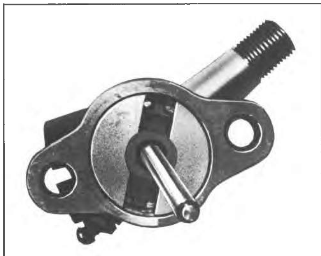
Fig. 3B-82--Proper Key Installation
