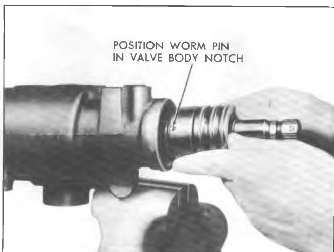
Fig. 3B-57--Valve to Worm Alignment
