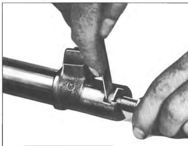
Fig. 3B-16—Checking Lash Adjuster End Clearance
