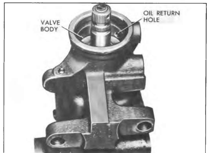
Fig. 3B-59--Valve Body Position in Housing
