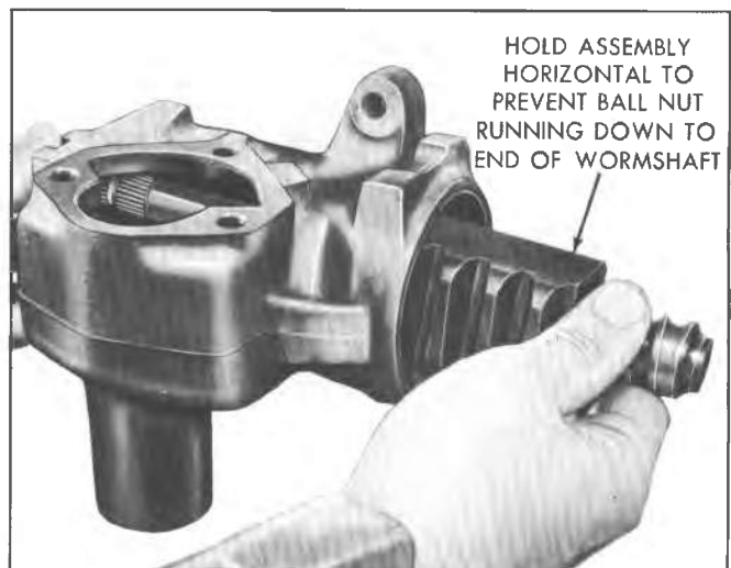
Fig. 3B-6--Removing the Wormshaft and Ball Nut--Typical
