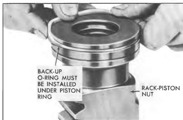
Fig. 3B-49--Installing Ring on Rack-Piston
