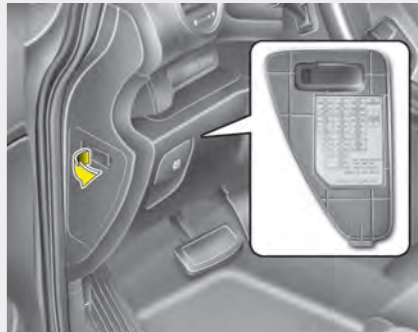
Inner fuse panel
