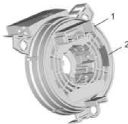
Fig. 17: Uplead Post And Centering Window Courtesy of GENERAL MOTORS COMPANY
