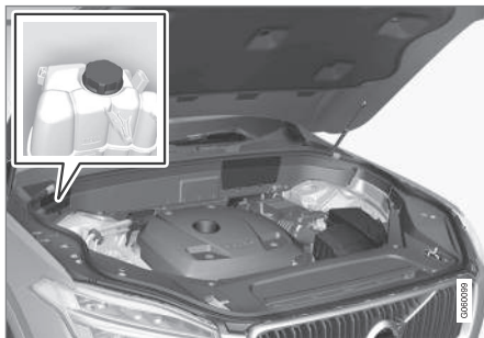
Coolant expansion tank
