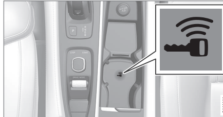
Back-up reader in the tunnel console
