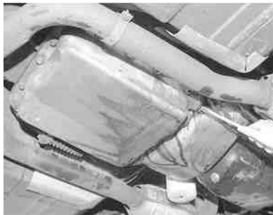
Fig. 3: Loosen the rear oil pan bolts about 4 turns, then carefully pry the front of the pan down, and allow the fluid to drain
