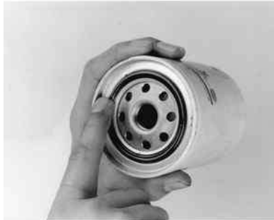
Fig. 9: Before installing a new oil filter, lightly coat the rubber gasket with clean oil
