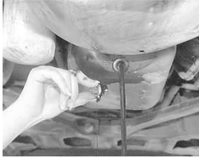
Fig. 4: Make sure you thoroughly clean the oil pan drain plug threads to avoid stripping the pan threads
