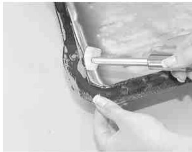
Fig. 9: Remove and discard the pan gasket, then use a suitable scraper to carefully clean the mating surfaces
