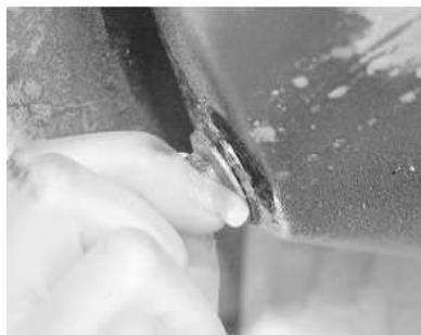
Fig. 2: Keep an inward pressure on the drain plug while loosening it, so hot oil does not drip onto your hands
