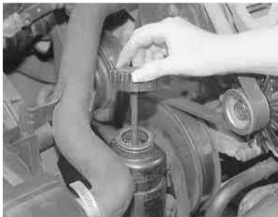
Fig. 2: Unscrew the power steering reservoir cap/dipstick
