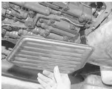
Fig. 7: Remove the transmission filter and seal
