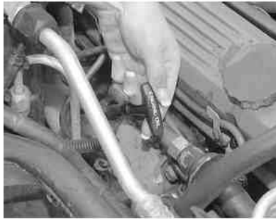
Fig. 1: Pull the dipstick out of the tube
