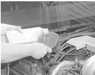
Fig. 3: Using a funnel, SLOWLY add a small amount of fluid through the dipstick tube, stopping often to check the level
