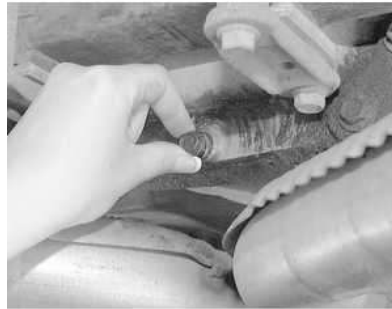
Fig. 2: After the drain plug has been loosened, you can unthread it by hand
