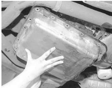
Fig. 5: Remove the remaining bolts, then carefully lower the pan and dump any remaining fluid in a suitable container
