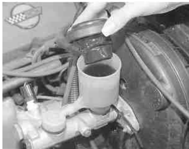
Fig. 3: Remove the master cylinder reservoir cap by pulling it off the top of the reservoir. Note the cap diaphragm
