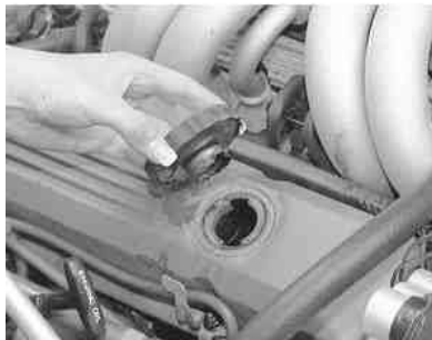
Fig. 3: If the level is low, remove the engine oil fill cap, located on the valve cover
