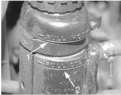
Fig. 1: The power steering fluid reservoir is marked with FULL HOT (1) and FULL COLD (2) lines
