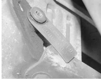
Fig. 1: The rear axle fill plug has tag on it listing the type of fluid required
