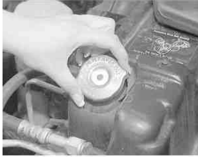
Fig. 1: NEVER take the radiator cap off when the engine is hot!
