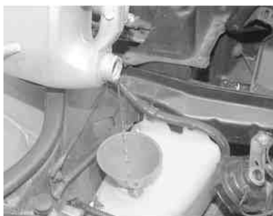
Fig. 6: If the fluid level is low, add coolant to the recovery reservoir until it reaches the proper level
