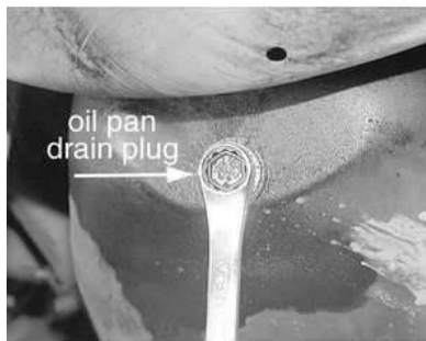
Fig. 1: Use a 13mm box-end wrench or ratchet to loosen the oil pan drain plug
