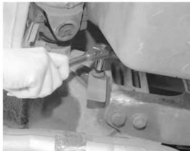
Fig. 2: Use a ratchet with a hex socket to loosen the filler plug
