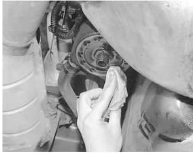
Fig. 8: Use a clean, lint-free rag to wipe off the engine block filter adapter
