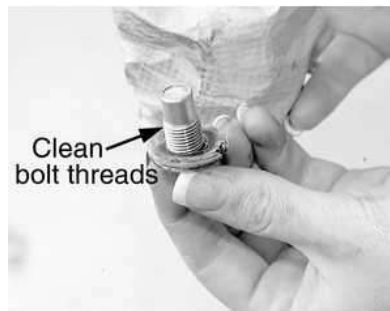
Fig. 4: Make sure you thoroughly clean the oil pan drain plug threads to avoid stripping the pan threads
