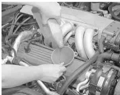
Fig. 4: Then, using a funnel, add the proper type and amount of oil
