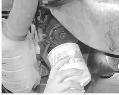
Fig. 7: Carefully lower the oil filter. Remember, it's holding about a quart of hot, dirty oil
