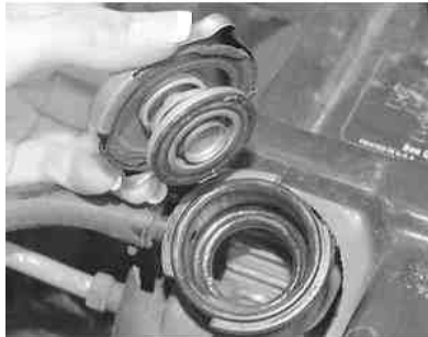
Fig. 2: When you remove the radiator cap, check the gaskets and make sure they are OK
