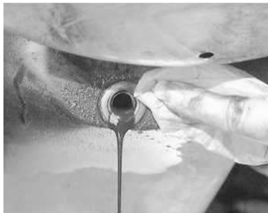
Fig. 5: Also, make sure to clean the oil pan drain plug mating surface
