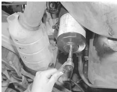
Fig. 6: You can use a cap-type oil filter wrench with a socket to loosen the oil filter
