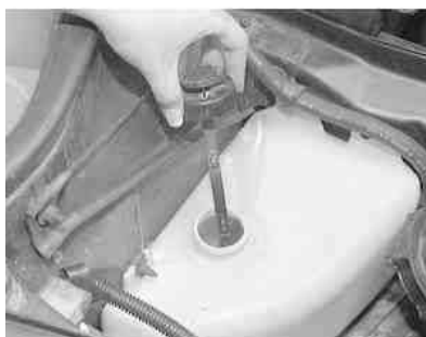
Fig. 5: If equipped, unscrew the reservoir cap/dipstick in order to get a fluid level reading
