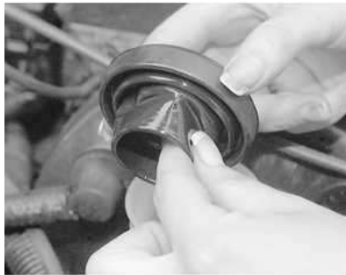
Fig. 5: If the cap diaphragm is extended due to low fluid levels . . .
