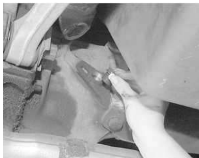
Fig. 3: Finish unscrewing the plug by hand, then remove it
