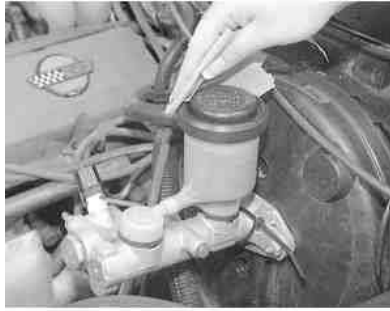
Fig. 1: Clean all of the dirt from the master cylinder cap, to avoid contaminating the system when you remove the cap
