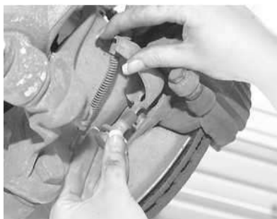
Fig. 6: Pull the bolts from the rear of the hub and bearing assembly
