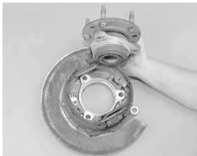
Fig. 9: You can pull the hub and bearing away from the backing plate
