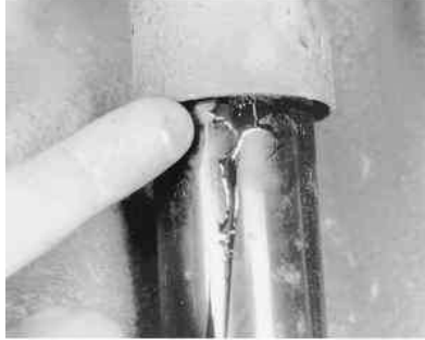
Fig. 1: When fluid is seeping out of the shock absorber, it's time to replace it
