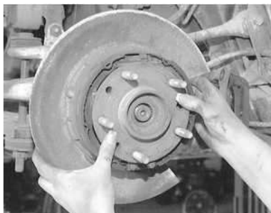
Fig. 7: Once the 3 bolts are removed, you can pull the hub and bearing, along with the backing plate off the driveshaft
