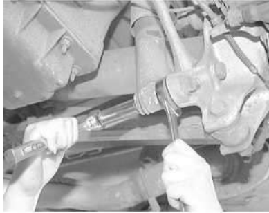
Fig. 1: While holding the nut stationary with a wrench, loosen the lower shock mounting bolt
