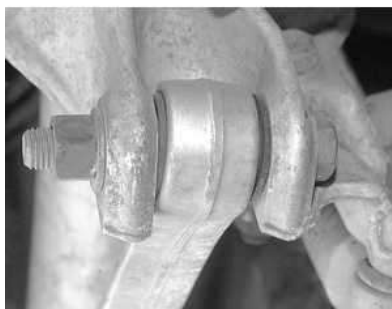
Fig. 3: The control rod is secured to the knuckle with a bolt and nut
