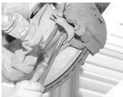
Fig. 5: Access to the hub and bearing Torx® bolts is difficult; you may have to turn the driveshaft and/or use an extension
