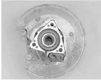
Fig. 9: You can pull the hub and bearing away from the backing plate
