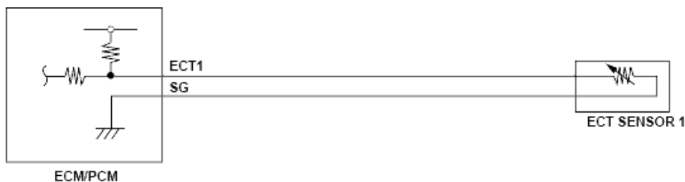
Fig. 11: Engine Coolant Temperature (ECT) Sensor 1 (Low Voltage) - Circuit Diagram
