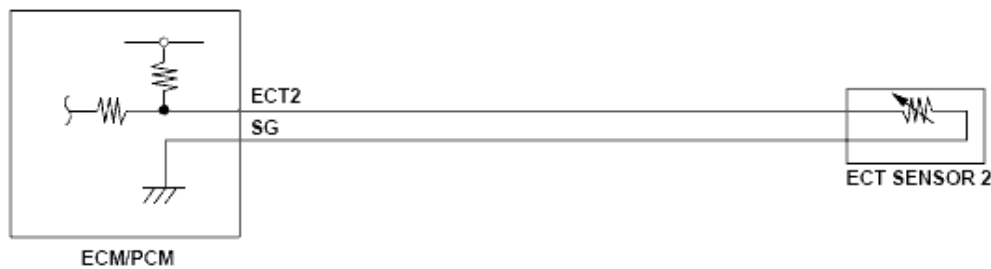
Fig. 271: Engine Coolant Temperature (ECT) Sensor 2 Circuit Diagram (Low Voltage)
