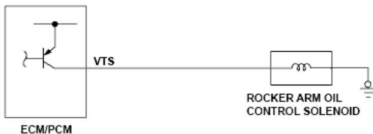
Fig. 315: Rocker Arm Oil Control Solenoid Circuit Diagram (High Voltage)
