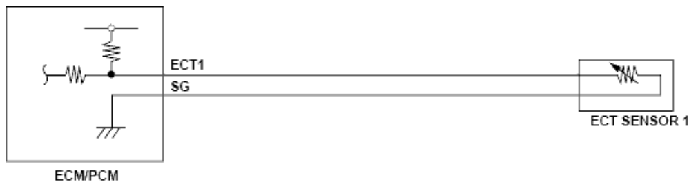
Fig. 13: Engine Coolant Temperature (ECT) Sensor 1 (High Voltage) - Circuit Diagram
