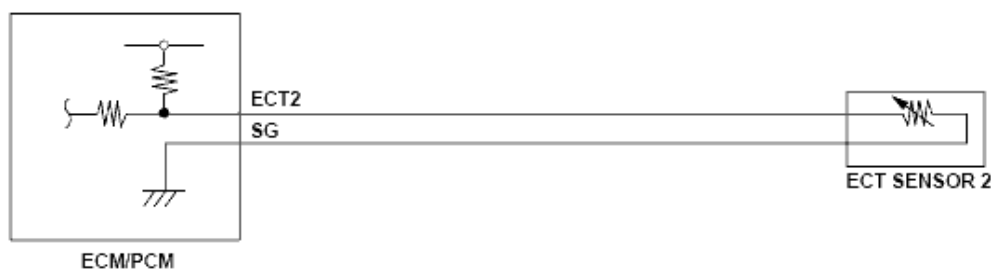
Fig. 273: Engine Coolant Temperature (ECT) Sensor 2 Circuit Diagram (High Voltage)
