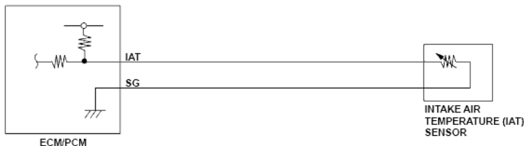
Fig. 6: Intake Air Temperature (IAT) Sensor (Low Voltage) - Circuit Diagram
