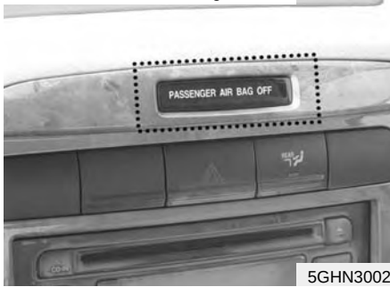
The location of OCS warning indicator
