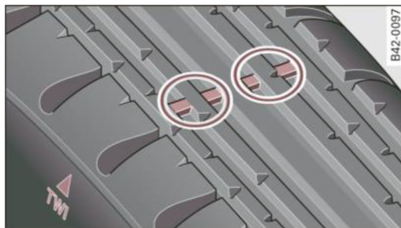
Fig. 125 Tire tread: tread wear indicators (TWI)
