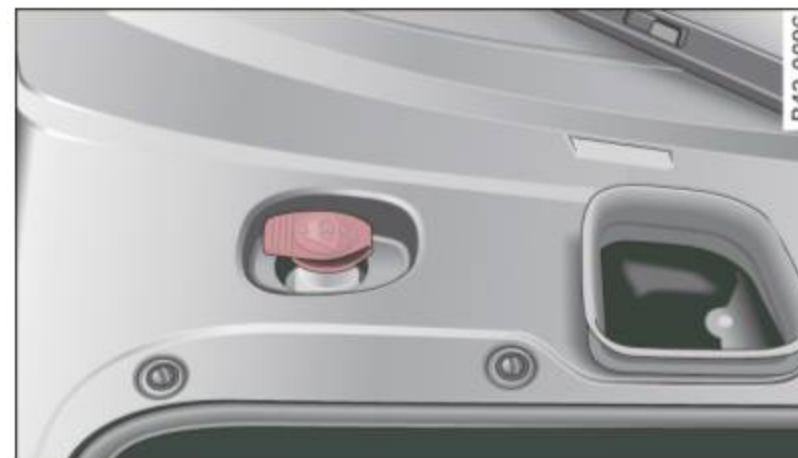
Fig. 122 Luggage compartment: Windshield washer fluid reservoir
