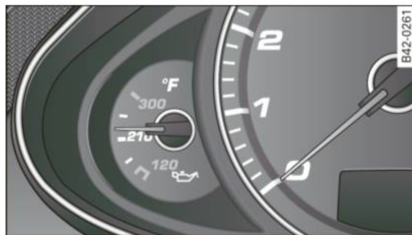
Fig. 118 Instrument cluster: Engine oil temperature display
