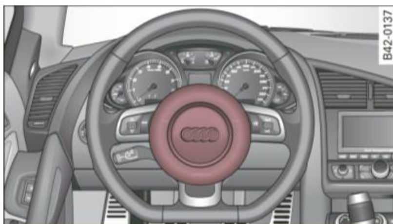
Fig. 97 Location of driver airbag: in steering wheel
