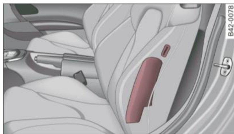
Fig. 103 Side airbag location in the driver's seat
