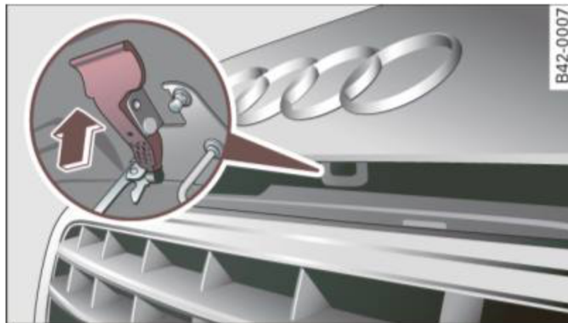
Fig. 37 Release lever under the front lid
