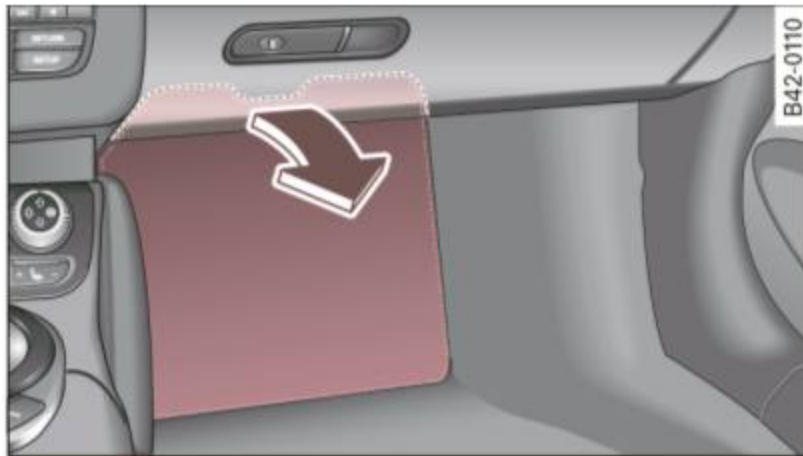
Fig. 137 Passenger's side wheel well: Foot rest with fuse arrangement
