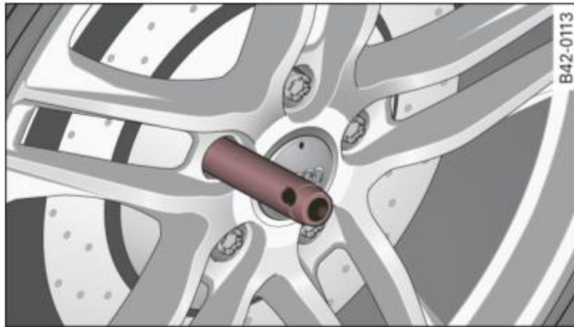
Fig. 134 Wheel change: alignment pin inside the top hole
