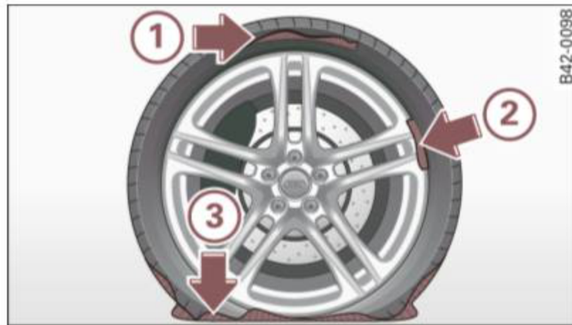
Fig. 128 Tire damage for which the Tire Mobility System is not suited
