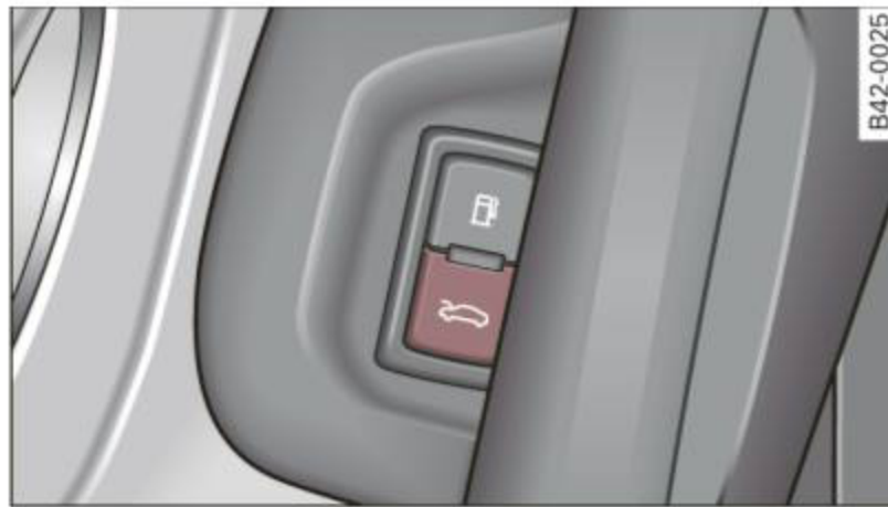
Fig. 36 Drivers door: remote front lid release
