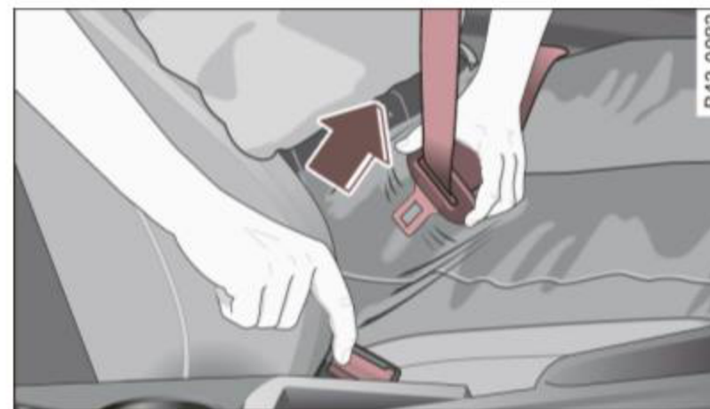
Fig. 96 Releasing the tongue from the buckle
