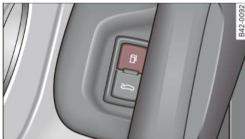
Fig. 112 Driver's door: Unlocking fuel filler flap
