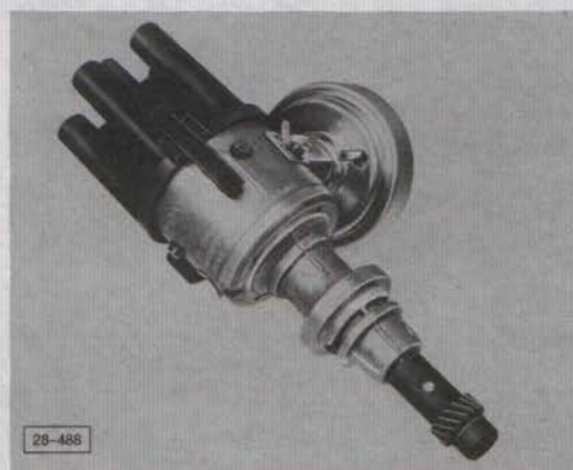
Hall TCI distributor for short cylinder head: for engines with code letters WC, Part No. 035 905 206
