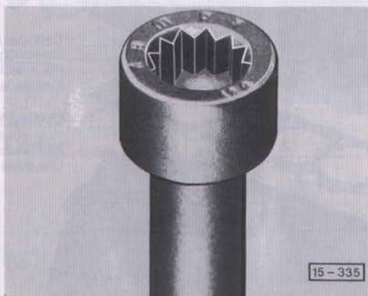
Fig. 2 Cylinder head bolts with 12 point socket head 12 point socket head bolts from Eng. No. WC 008 993, WE, WG, WJ
