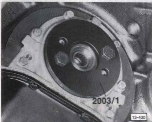
Fig. 9 Installing oil seal, flywheel end
