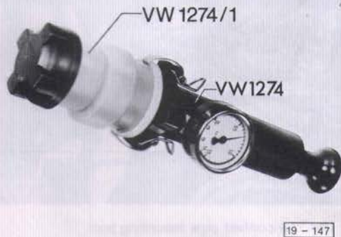
Fig. 2 Checking pressure relief valve in cap
