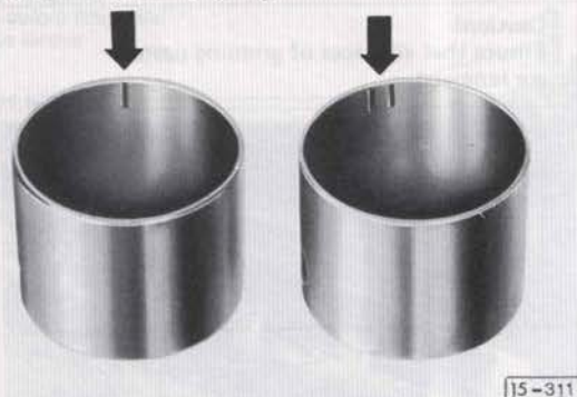
Fig. 9 Mark tappets on removal
