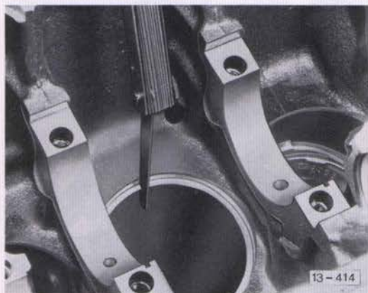
Fig. 8 Measuring ring gap
