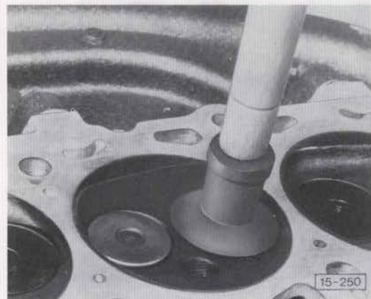
Fig. 5 Grinding valves in
