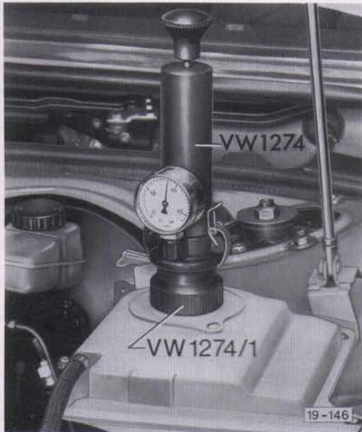
Fig. 1 Checking cooling system for leaks
