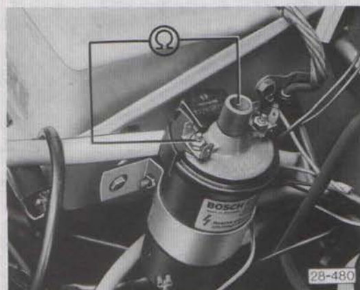
Fig. 2 Checking secondary resistance of ignition coil
