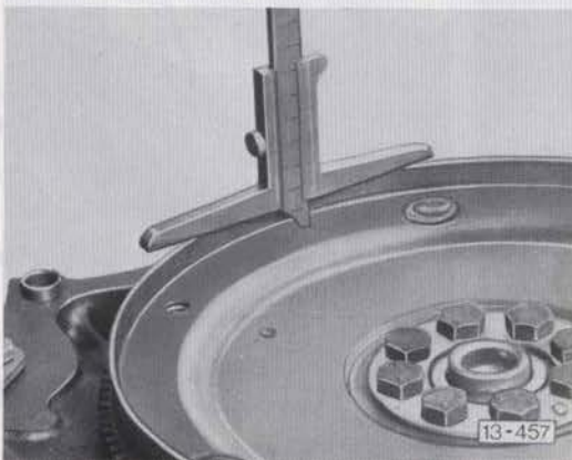
Fig. 3 Measuring distance from drive plate, inside
