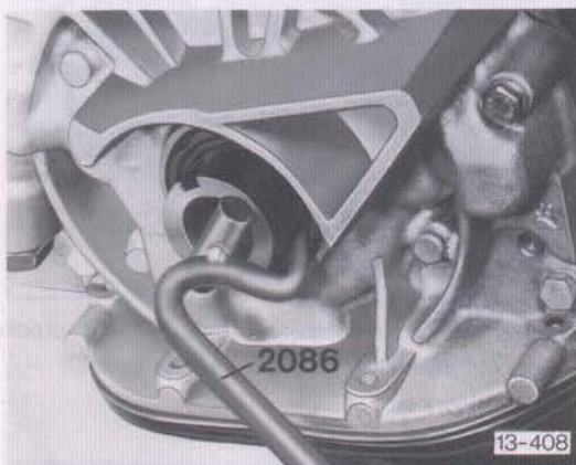
Fig. 7 Levering out crankshaft oil seal at pulley end
