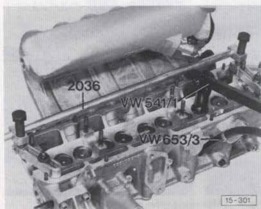
Fig. 7 Removing valve cotters
