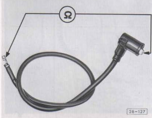
Fig. 3: Checking ignition leads
