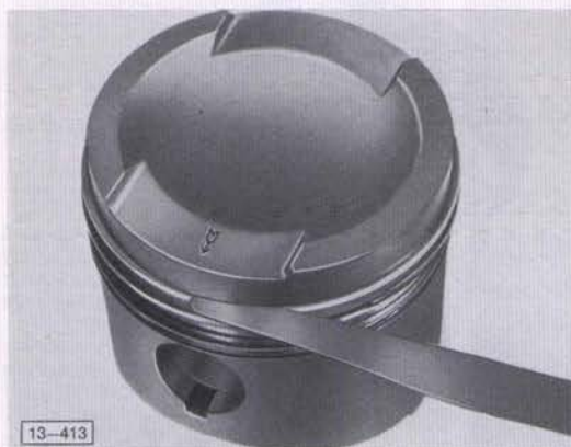
Fig. 7 Measuring ring clearance
