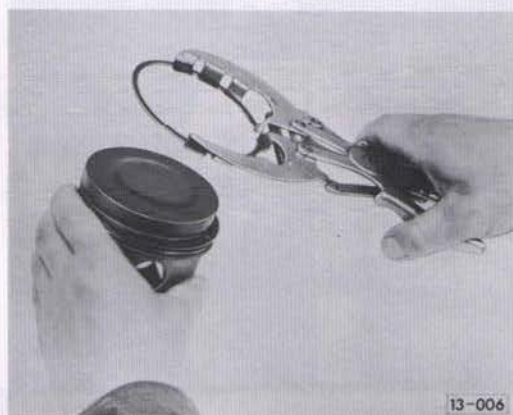
Fig. 10 Removing and installing rings
