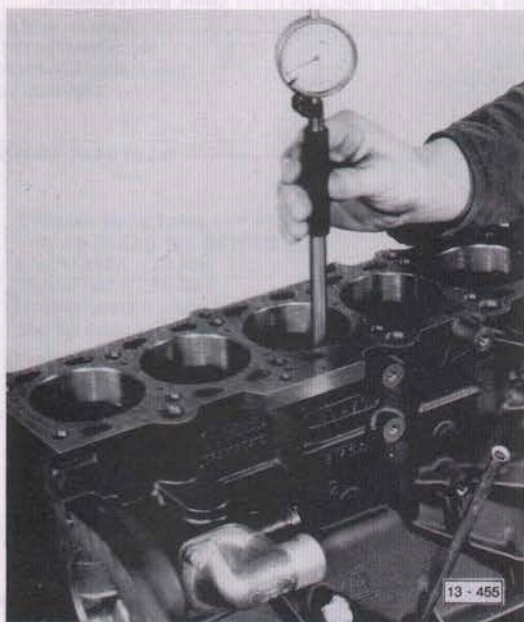
Fig. 13 Measuring bores — Measure with internal dial gauge
