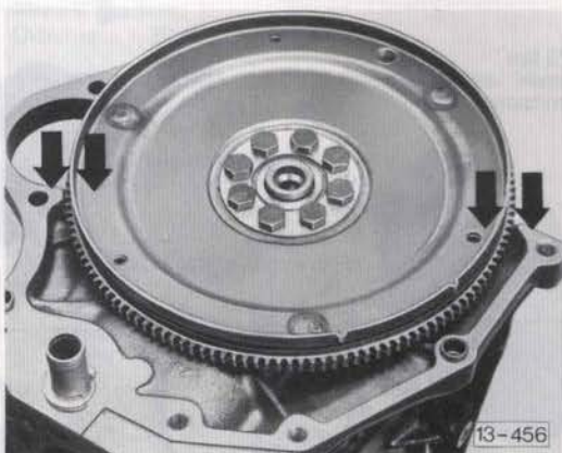
Fig. 5 Measure distance from drive plate to engine block in two places
