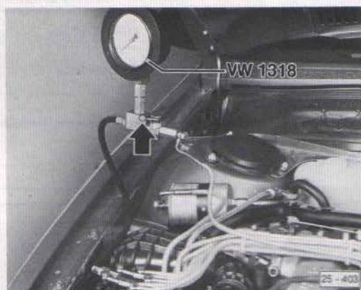
Fig. 3 Pressure gauge valve in closed position
