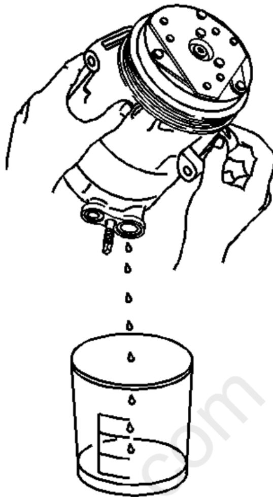
Fig. 4: Draining A/C Refrigerant Oil From Compressor Courtesy of GENERAL MOTORS COMPANY
