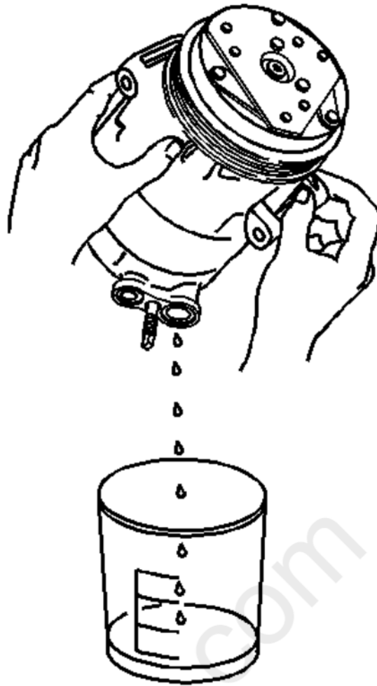
Fig. 3: Draining A/C Refrigerant Oil From Compressor Courtesy of GENERAL MOTORS COMPANY
