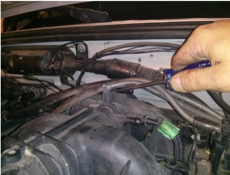
Unbolt the Ignition Wire Flange Mount.
