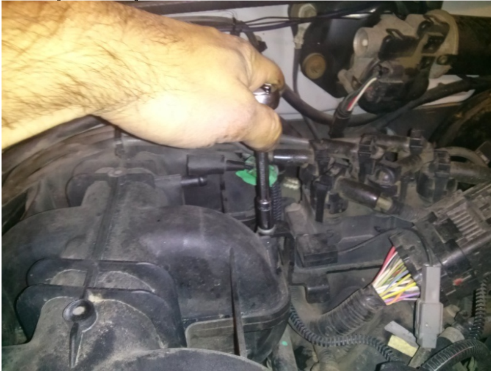
Unbolt the Ignition Wire Flange Mount.
