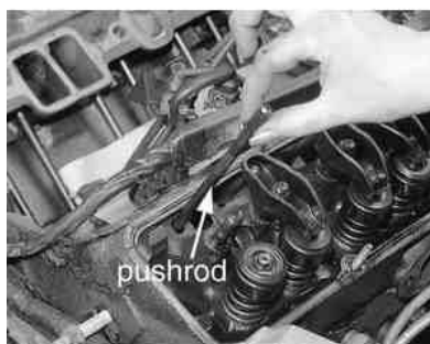
Fig. 8: Then, pull the pushrods from the cylinder head
