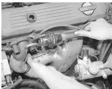
Fig. 7: You will probably have to move the check valve pipe aside in order to remove the exhaust manifold
