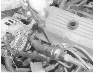
Fig. 4: . . . then disconnect the AIR hose from the exhaust check valve
