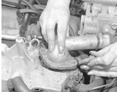
Fig. 6: If necessary, unfasten the mounting bolts and remove the coolant outlet
