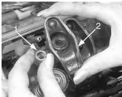
Fig. 7: Remove the rocker arm retaining nut (1) and rocker arm (2)
