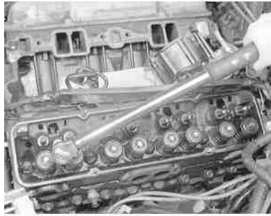
Fig. 13: Always use a torque wrench to tighten the cylinder head bolts to specifications
