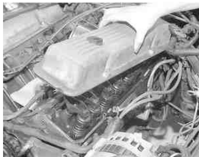
Fig. 4: Remove the rocker arm (valve) cover
