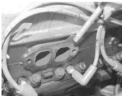
Fig. 9: Also, make sure to thoroughly clean the head-to-manifold mating surfaces
