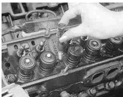
Fig. 10: When you remove the cylinder head bolts, keep them in order, because 2 different lengths of bolts are used
