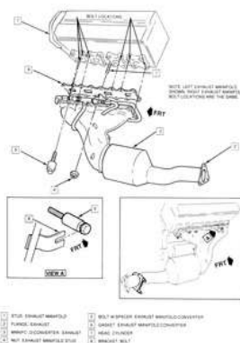
Fig. 10: The exhaust manifold/converter assembly is removed as a single unit — 1990–91 and early 1992 5.7L (VIN J) engine
