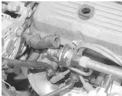
Fig. 4: . . . then disconnect the AIR hose from the exhaust check valve
