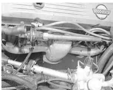
Fig. 6: Top view of the exhaust manifold, after the pipe is disconnected
