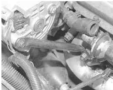
Fig. 5: The rear alternator brace is secured with a bolt at the top and a nut at the bottom
