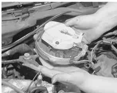
Fig. 3: Remove the distributor from the engine
