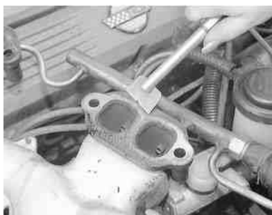
Fig. 8: Use a scraper to carefully clean the mating surfaces of the manifold
