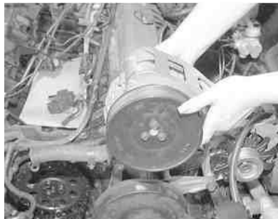
Fig. 3: Unfasten the retainers, then remove the AIR pump and bracket, as an assembly, from the engine
