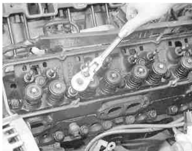
Fig. 10: When you remove the cylinder head bolts, keep them in order, because 2 different lengths of bolts are used
