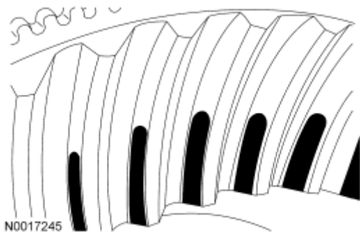
Fig. 7: Identifying Tooth Contact Pattern (Thick Contact Pattern - Toe) Courtesy of FORD MOTOR CO.
