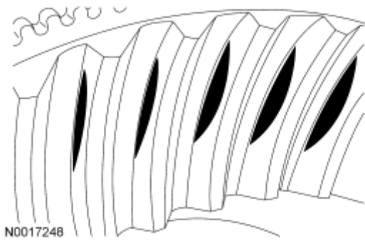
Fig. 5: Identifying Tooth Contact Pattern (High, Thin Contact Pattern) Courtesy of FORD MOTOR CO.
