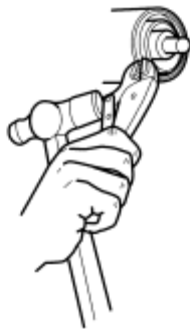
Fig. 18: Removing Drive Pinion Seal Courtesy of FORD MOTOR CO.
