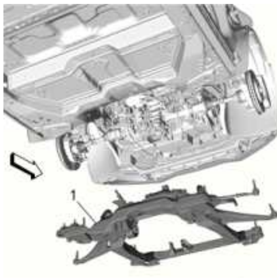
Fig. 33: Drivetrain And Front Suspension Cradle Courtesy of GENERAL MOTORS COMPANY
