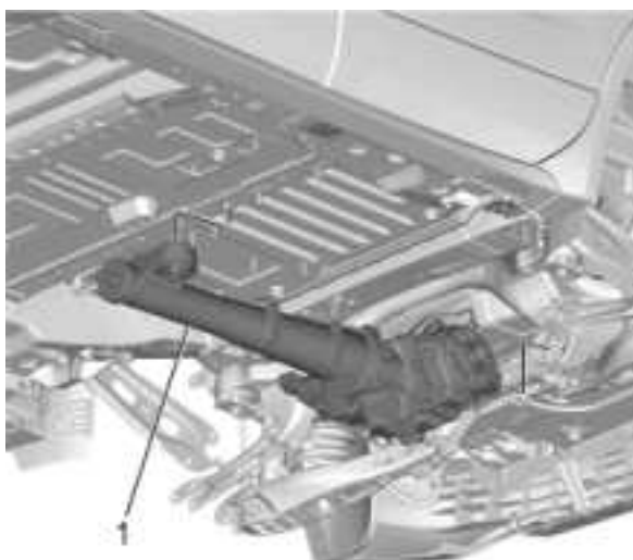
Fig. 53: Rear Differential Assembly Courtesy of GENERAL MOTORS COMPANY
