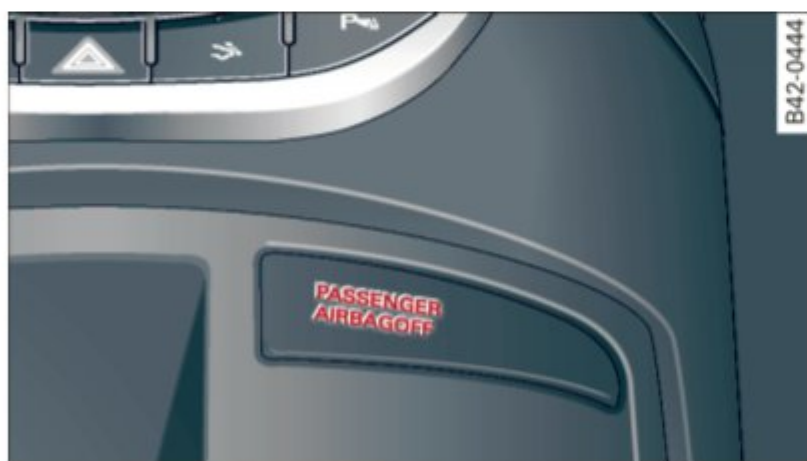
Fig. 120 Section from the instrument panel: PASSENGER AIR BAG OFF light
