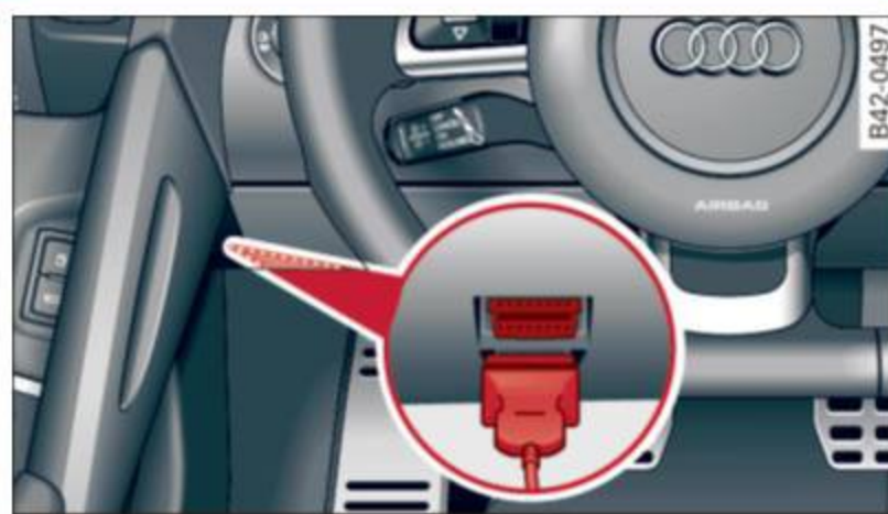
Fig. 19 Location of Data Link Connector (DLC)
