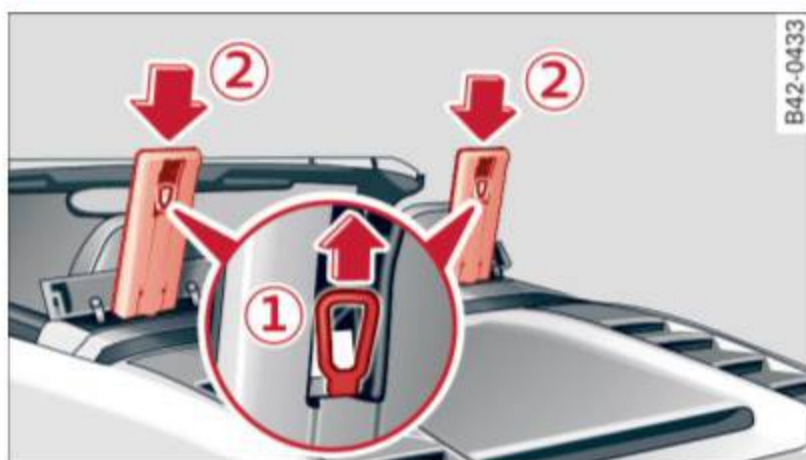
Fig. 106 Deployed rollbar with release loop
