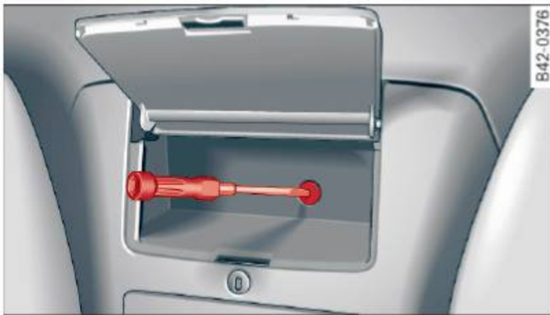
Fig. 37 Upper storage compartment: removing the cover
