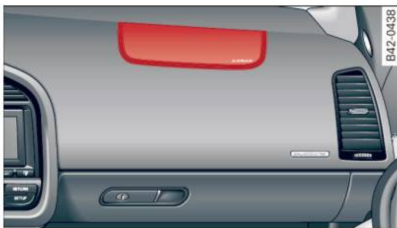
Fig. 118 Location of front passenger's airbag: in the instrument panel
