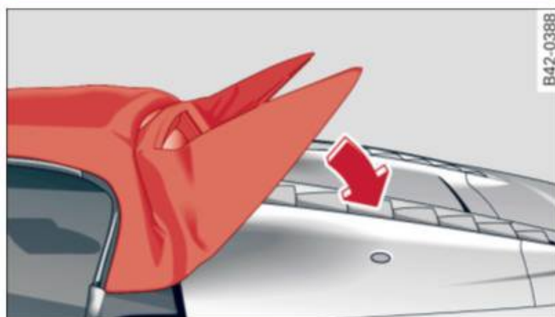
Fig. 49 Convertible top: pressing the fins downward
