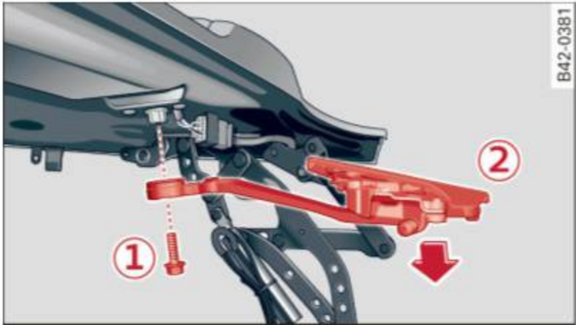
Fig. 42 Convertible top storage bay lid: removing the cover
