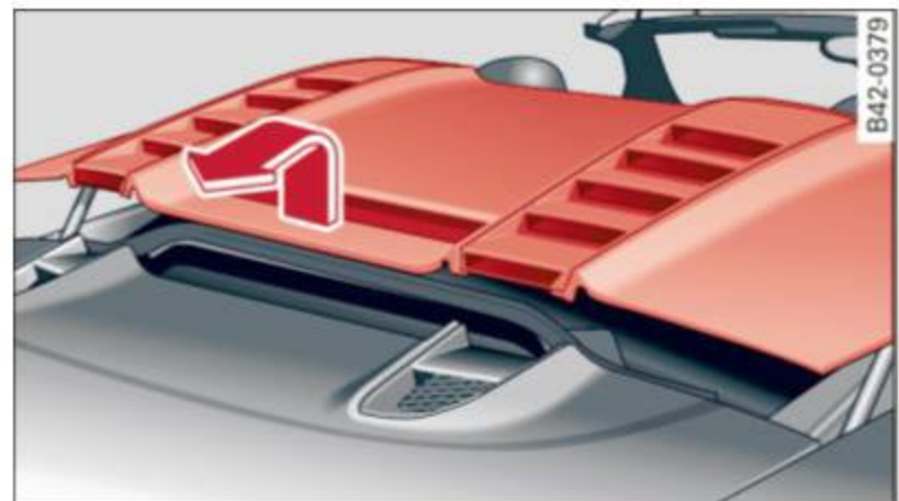
Fig. 40 Raising the storage bay lid and pulling it back
