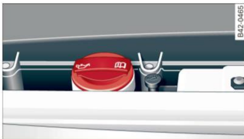
Fig. 142 Engine compartment: Oil filler cap location
