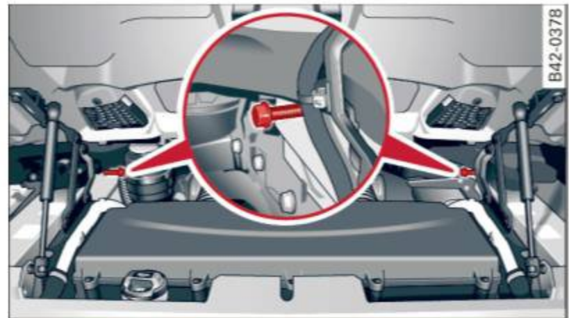
Fig. 39 Engine compartment: installing the emergency operation bolts
