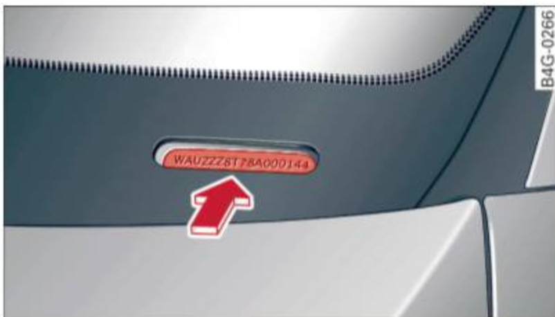
Fig. 168 Vehicle Identification Number (VIN) plate: location on driver's side dash panel
