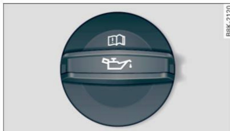
Fig. 143 Engine compartment: cover on the engine oil filler neck
