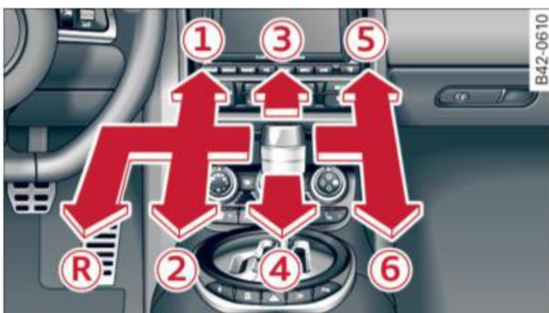
Fig. 82 Gearshift pattern: 6-speed manual transmission
