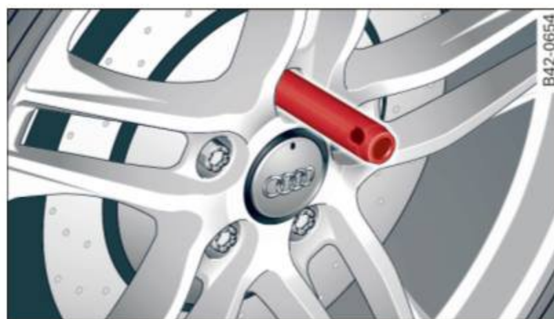
Fig. 162 Wheel change: alignment pin inside the top hole
