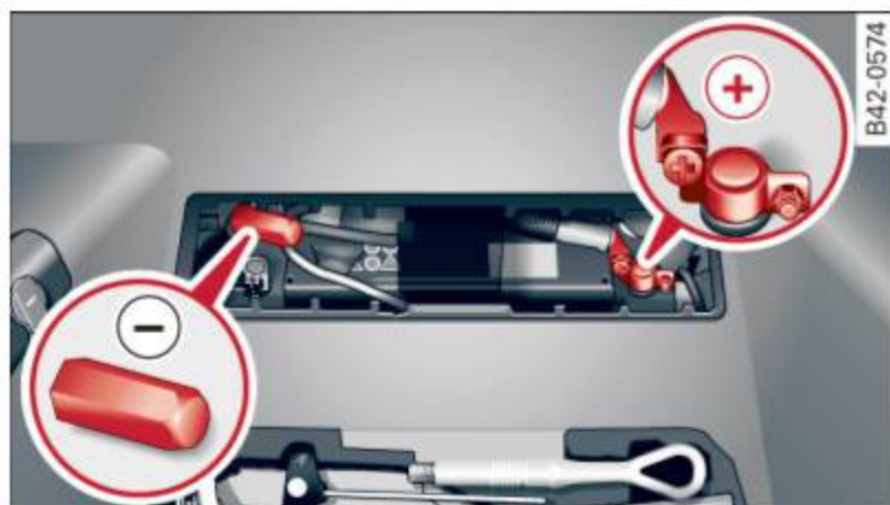
Fig. 147 Luggage compartment: connectors for a charger and jump start cables
