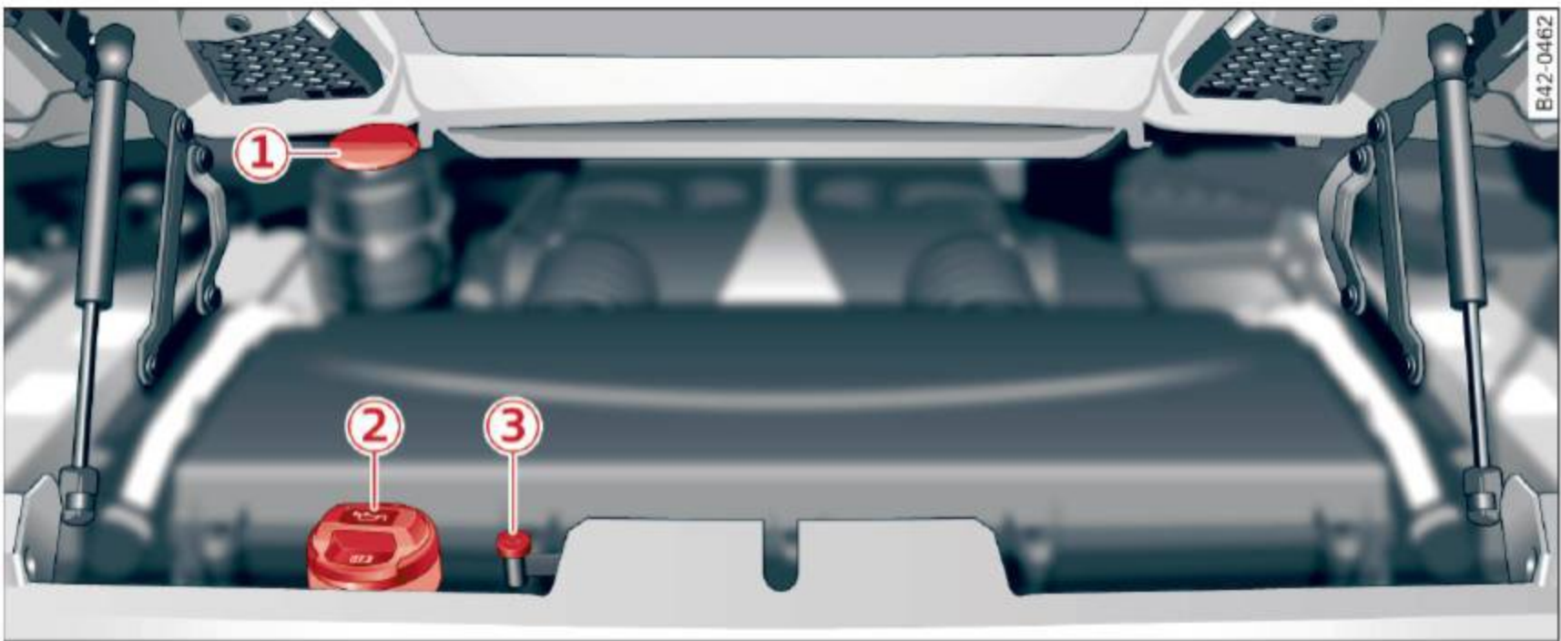
Fig. 136 Typical layout for containers, engine oil dipstick and engine oil filler cap (manual transmission)
