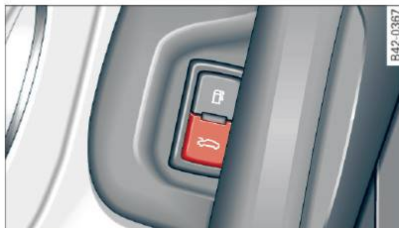
Fig. 27 Drivers door: remote front lid release
