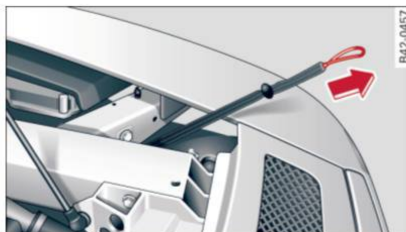
Fig. 133 Engine compartment: releasing the fuel filler flap using the emergency release
