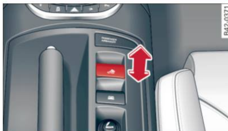
Fig. 32 Center console: convertible top switch
