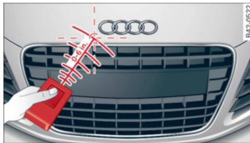
Fig. 100 Front bumper: location of transmitter unit
