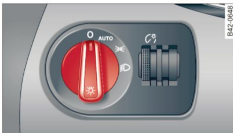
Fig. 52 Instrument panel: light switch (automatic head- and taillight control)
