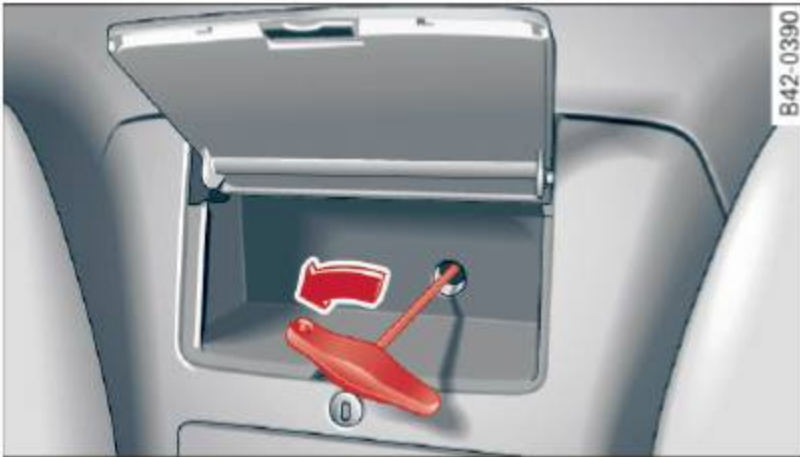
Fig. 51 Upper storage compartment between the seat backrests: extending the rear window
