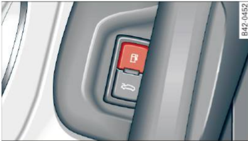
Fig. 130 Driver's door: Unlocking fuel filler flap
