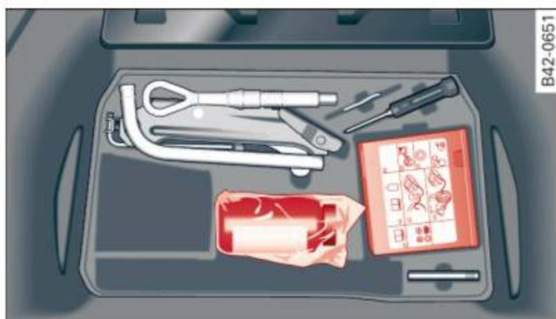
Fig. 155 Tire Mobility System under luggage compartment floor
