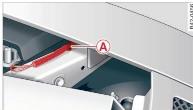
Fig. 132 Engine compartment: loosening the fuel filler flap cable
