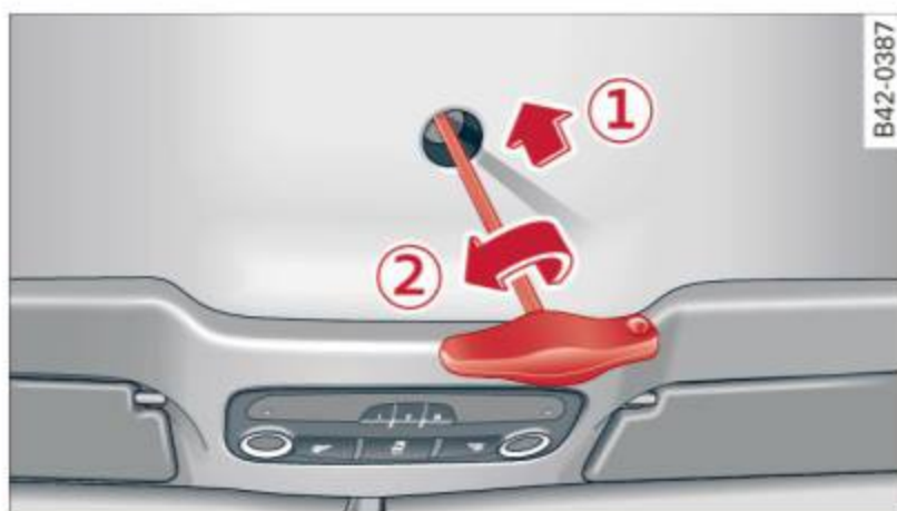
Fig. 48 Inner side of the convertible top: positioning the Allen wrench
