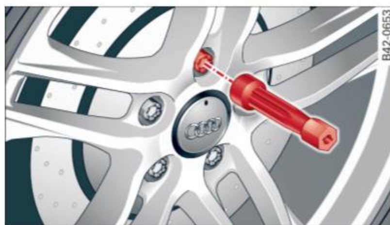
Fig. 161 Wheel change: using the screwdriver handle (with the blade removed) to turn the bolts
