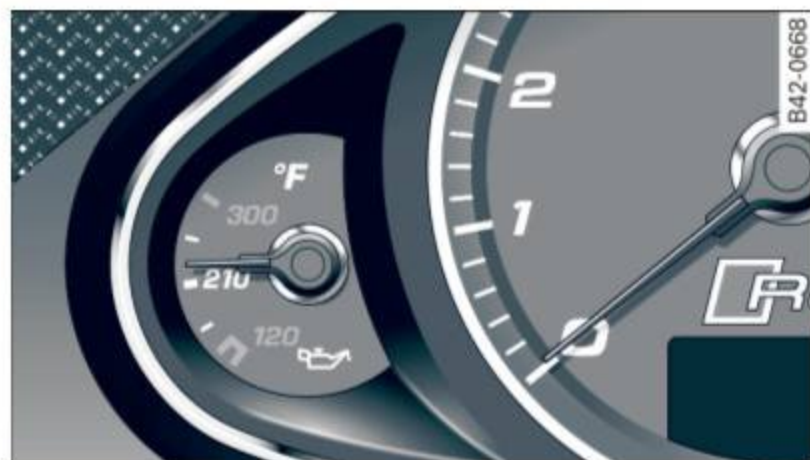
Fig. 140 Instrument cluster: Engine oil temperature display
