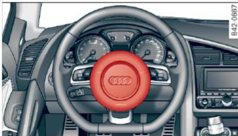
Fig. 117 Location of driver airbag: in steering wheel
