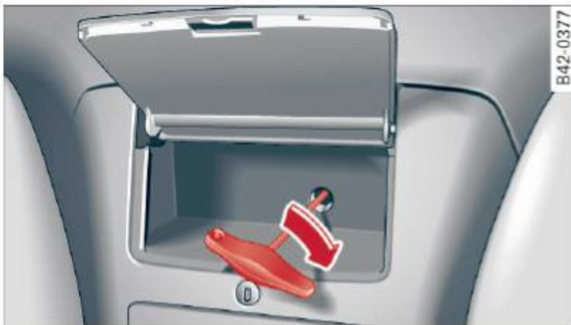
Fig. 38 Upper storage compartment: using the Allen wrench as a crank to lower the rear window
