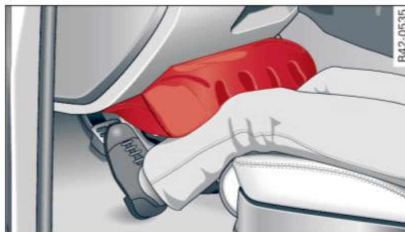
Fig. 122 Inflated airbags protecting in a frontal collision
