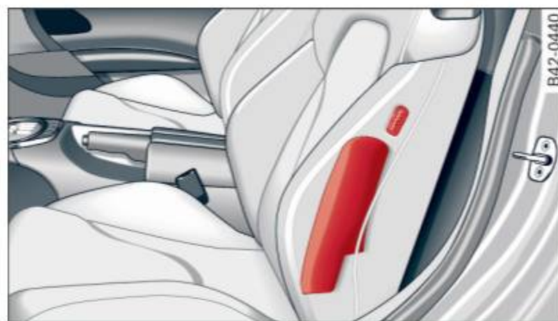
Fig. 123 Side airbag location in the driver's seat
