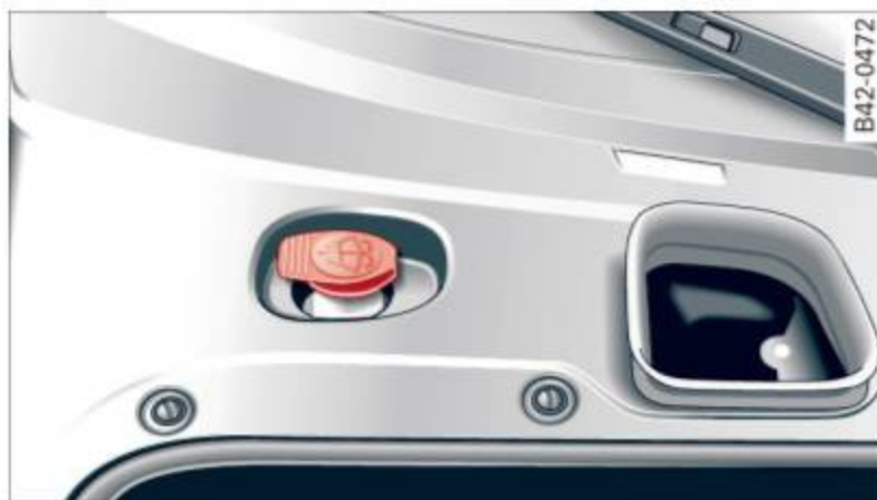
Fig. 148 Luggage compartment: Windshield washer fluid reservoir
