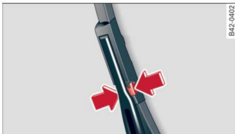
Fig. 61 Unlatching wiper blades
