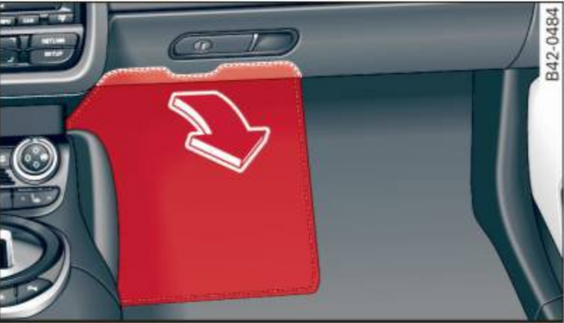
Fig. 166 Passenger's side wheel well: Foot rest with fuse arrangement
