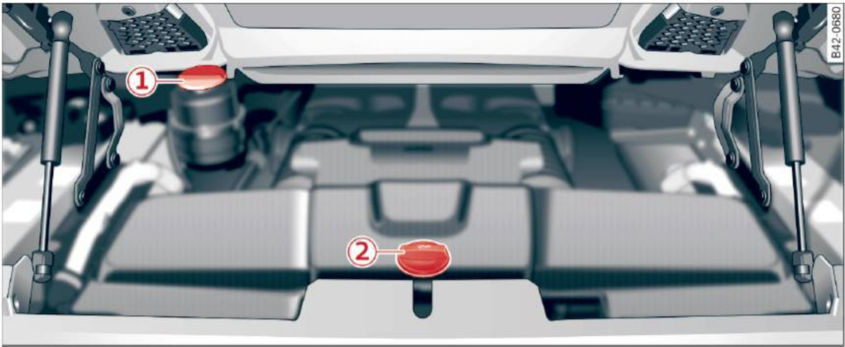
Fig. 137 Typical layout for containers, engine oil dipstick and engine oil filler cap (S tronic)
