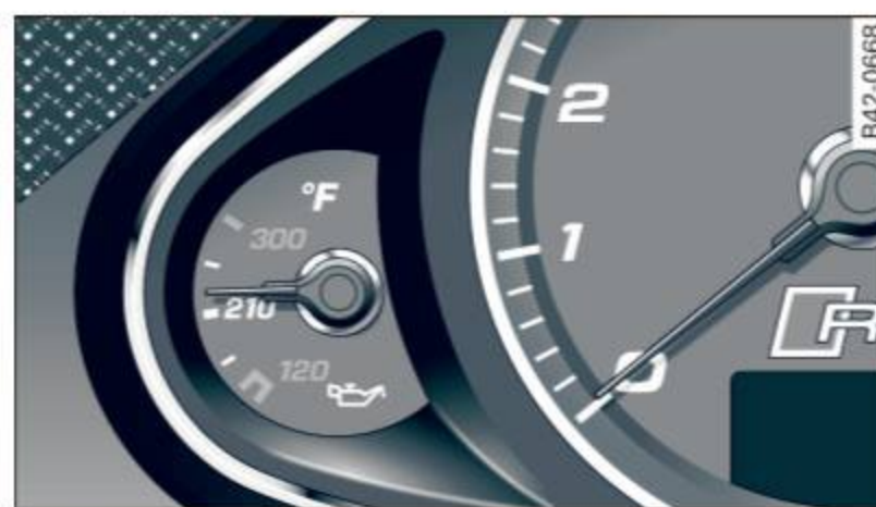
Fig. 138 Instrument cluster: Engine oil temperature display
