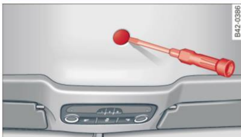
Fig. 47 Inner side of the convertible top: removing the cap
