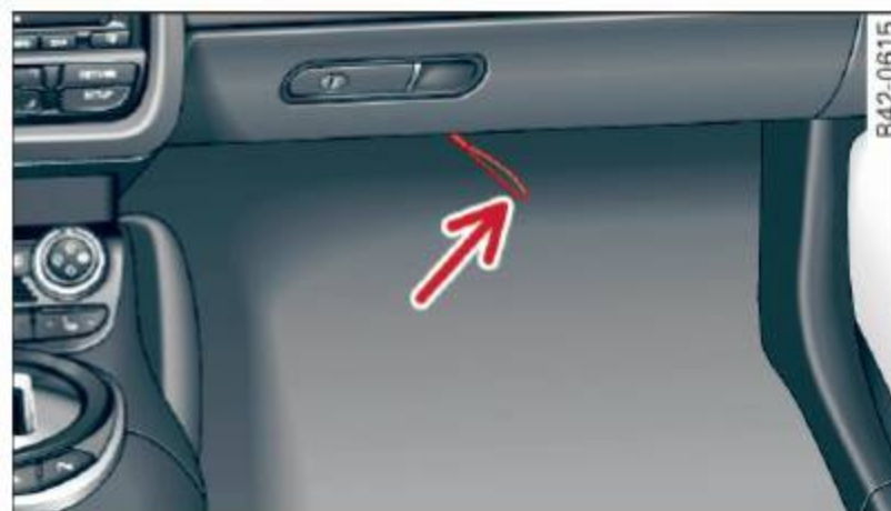
Fig. 29 Section: Emergency release
