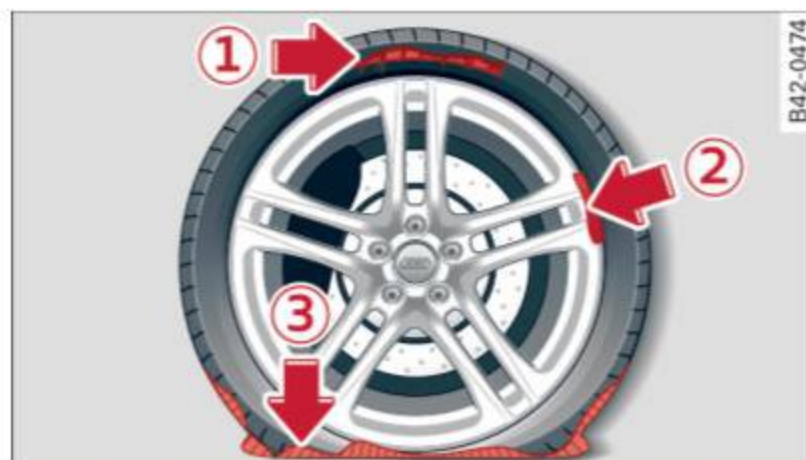
Fig. 154 Tire damage for which the Tire Mobility System is not suited
