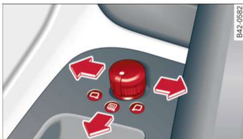
Fig. 57 Forward section of driver's armrest: power mirror controls
