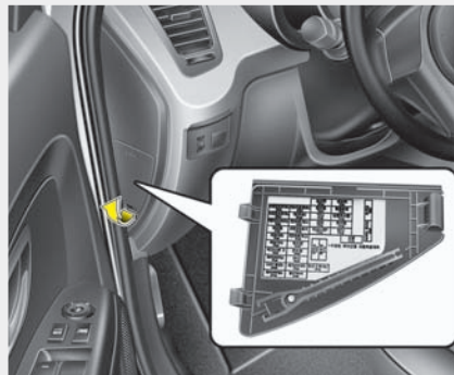
Inner fuse panel
