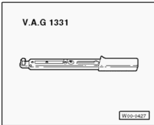
Fig. 22: Identifying Torque Wrench V.A.G. 1331 Courtesy of VOLKSWAGEN UNITED STATES, INC.
