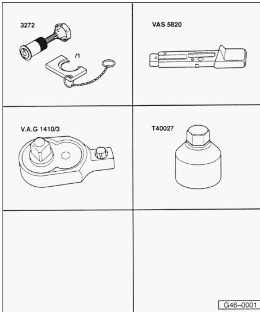
Fig. 103: Identifying Special Tools - Brake Pads, Removing And Installing Courtesy of VOLKSWAGEN UNITED STATES, INC.
