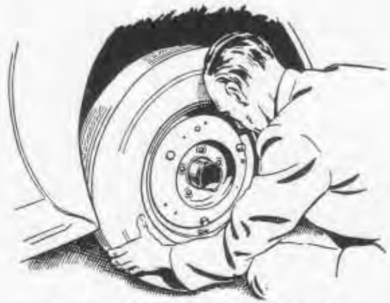
Fig. 27.—POSITIONING REAR WHEEL.
