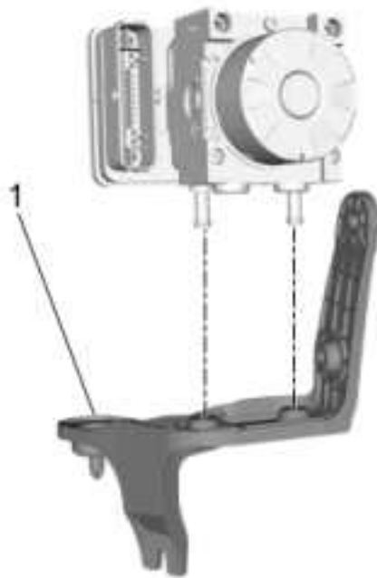
Fig. 22: Brake Pressure Modulator Valve Bracket Courtesy of GENERAL MOTORS COMPANY
