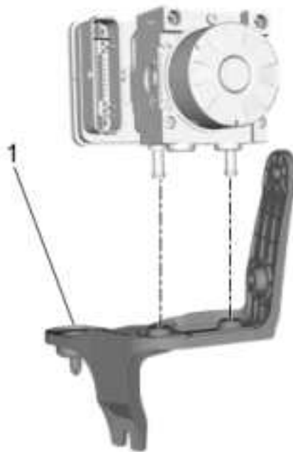
Fig. 21: Brake Pressure Modulator Valve Bracket Courtesy of GENERAL MOTORS COMPANY
