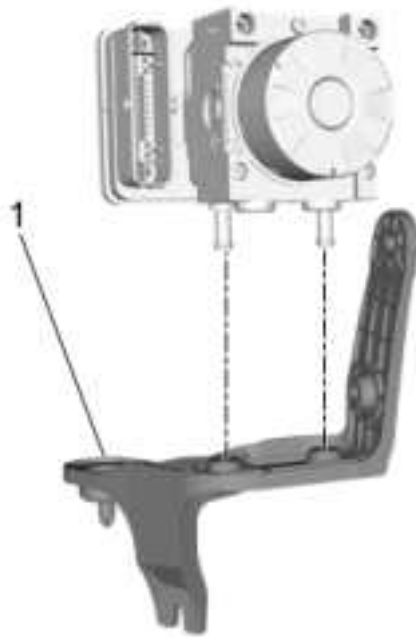
Fig. 37: Brake Pressure Modulator Valve Bracket Courtesy of GENERAL MOTORS COMPANY
