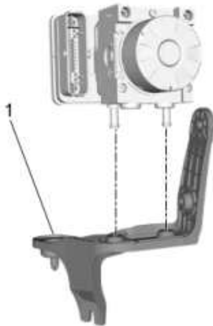
Fig. 38: Brake Pressure Modulator Valve Bracket Courtesy of GENERAL MOTORS COMPANY
