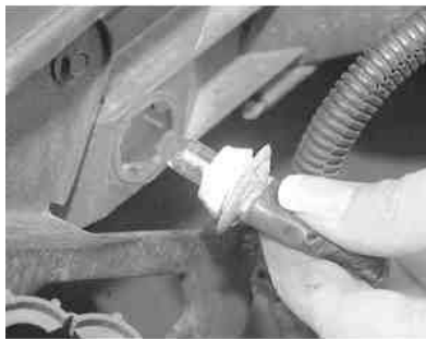
Fig. 4: To remove the side marker light bulb, twist the socket to unlock it, then pull it from the housing
