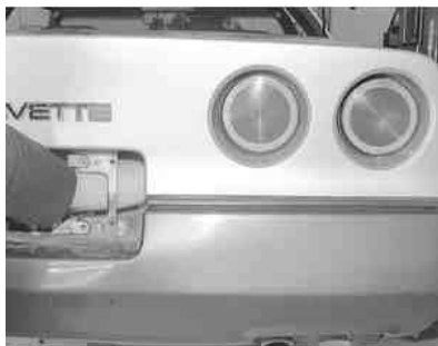
Fig. 8: Then, pull it out of the side and replace the bulb
