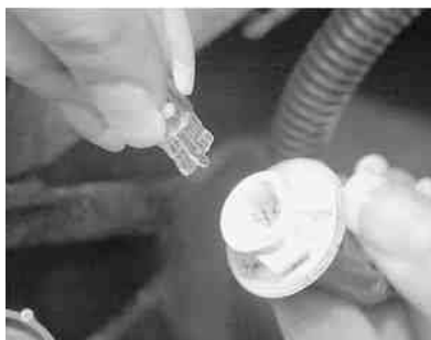
Fig. 5: Then, simply pull the bulb straight out of the socket
