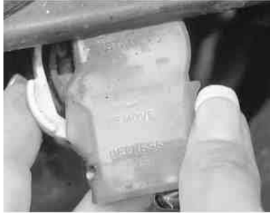
Fig. 1: You must depress the side tab, then rotate the socket and bulb assembly in the direction shown on the socket
