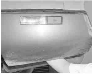
Fig. 10: To remove the rear side marker light, reach up from underneath the vehicle, depress the tab and rotate the bulb and socket
