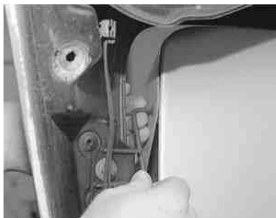
Fig. 1: With the hood in the raised position, unfasten the Torx® screws from the outer side of the headlight bezel/trim piece
