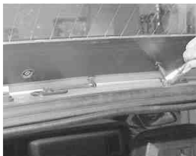
Fig. 12: Open the hatch, then unfasten the center high mount light 2 Torx® retaining screws
