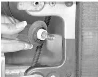
Fig. 23: Reach behind the license plate mounting and pull the reverse light bulb and socket out
