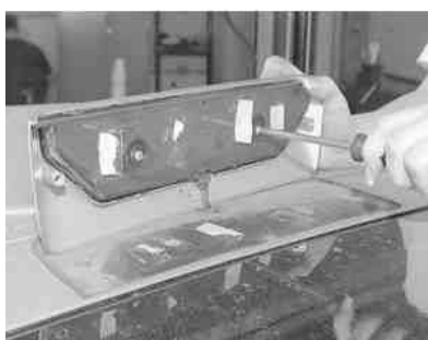
Fig. 14: Remove the retaining screws located on the under side of the 3rd brake light
