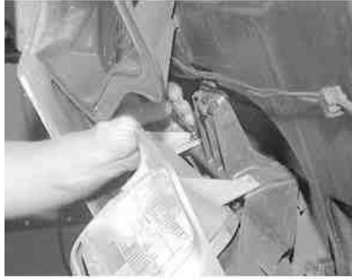
Fig. 5: Lift the bezel/trim piece away from the headlight assembly
