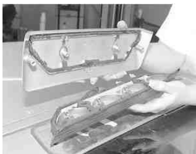
Fig. 15: Lift the cover for access to the bulbs. If you have to pry around the edges to remove it, be very careful
