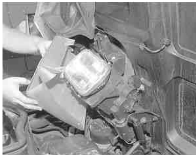
Fig. 5: Lift the bezel/trim piece away from the headlight assembly
