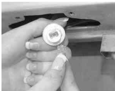
Fig. 22: The bulb can be pulled straight out of the socket for replacement
