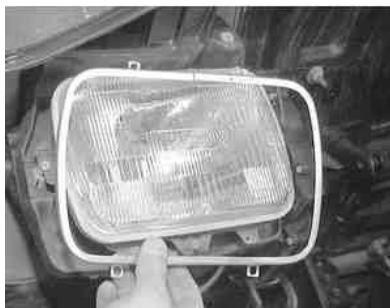
Fig. 7: Remove ONLY the 4 retaining ring screws, do NOT touch the aiming screws
