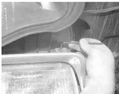
Fig. 4: ... then remove the remaining Torx® screw
