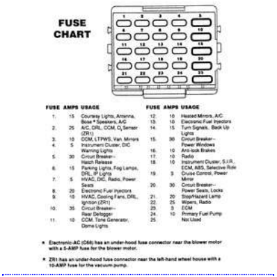
Fig. 25: Typical fuse identification
