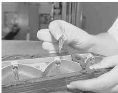
Fig. 16: When removing or installing bulbs, be careful not to bend the pins
