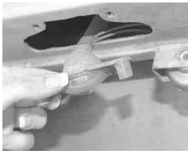
Fig. 20: After removing the retainers, pull the license plate lamp down
