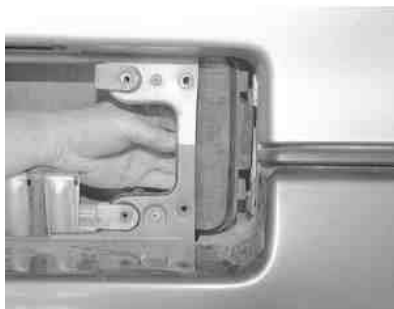
Fig. 8: Then, pull it out of the side and replace the bulb
