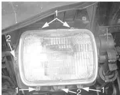
Fig. 6: With the hood closed, you can see the 4 headlight retaining ring screws (1) and 2 aiming screws (2)
