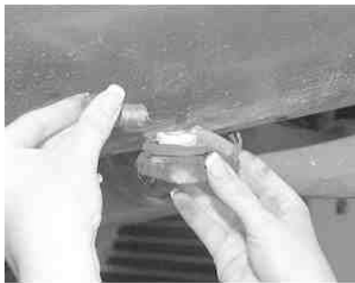
Fig. 11: Pull the bulb and socket down, turn the bulb to align the nubs with the channels in the socket, then pull the bulb out of the socket
