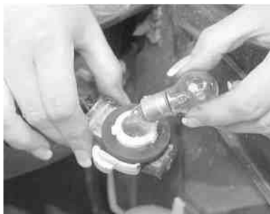
Fig. 3: Turn the bulb to align the nubs on the bulb with the channels in the socket, then carefully pull the bulb from the socket
