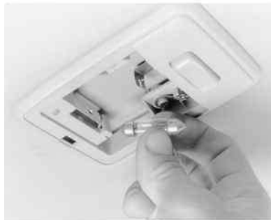
Fig. 18: Disengage the spring clip which retains one tapered end of this dome light bulb, then withdraw the bulb
