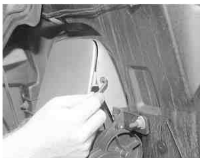
Fig. 2: You must then remove the screws from the inner side of the bezel/trim piece
