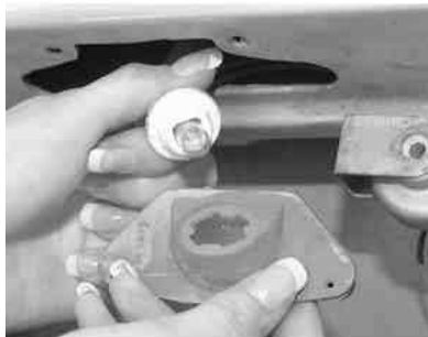
Fig. 21: Rotate the socket \frac{1}{4} turn to unlock it, then pull it out of the lens
