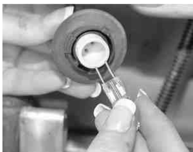
Fig. 24: Then, carefully pull the bulb straight out of the socket
