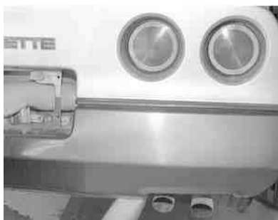
Fig. 6: To remove the inner rear brake light, you must reach behind the license plate and under the vehicle to access the bulb and socket
