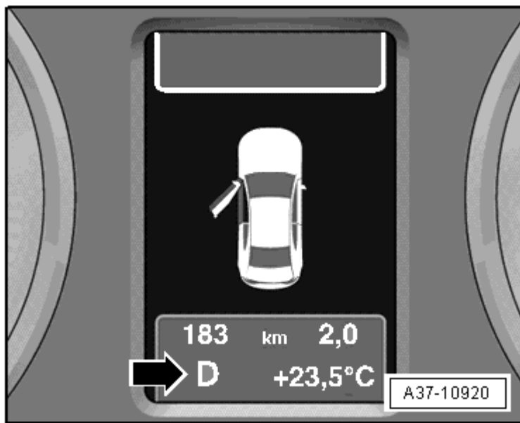
Fig. 34: Transmission Range Display -Y6- Courtesy of AUDI OF AMERICA, LLC
