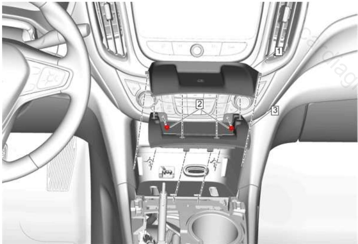
Fig. 21: Wireless Charging System Module Bracket Courtesy of GENERAL MOTORS COMPANY
