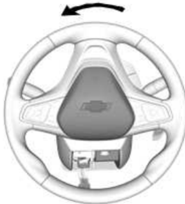
Fig. 14: Steering Wheel Rotated 180 Degrees To Left Courtesy of GENERAL MOTORS COMPANY
