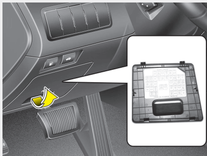
Instrument panel fuse panel
