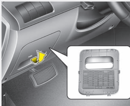
Inner fuse panel
