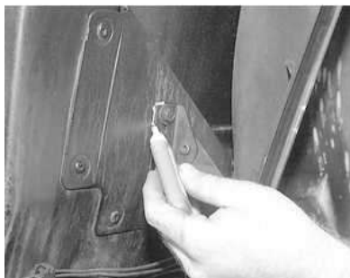
Fig. 3: All the hood hinges should be matchmarked before removal to assure proper alignment during installation
