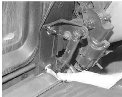
Fig. 2: Use a paint marker or equivalent to matchmark the lower hinge position
