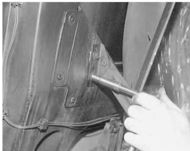
Fig. 6: It's very important to have the hood proper supported when removing the retaining bolts
