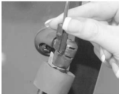
Fig. 1: To remove the hatch lid struts, detach the electrical connector
