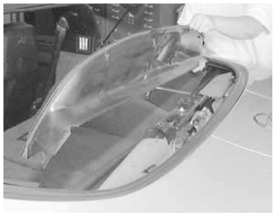
Fig. 7: If necessary, you can unfasten the retainers, remove the trim cover . . .
