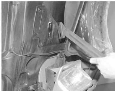
Fig. 7: With the help of an assistant, carefully pull the hinge away, then remove the hood from the vehicle
