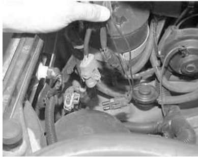
Fig. 1: Tag and detach any necessary electrical connectors for hood removal
