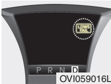
Lane departure warning system malfunction indicator (if equipped)
