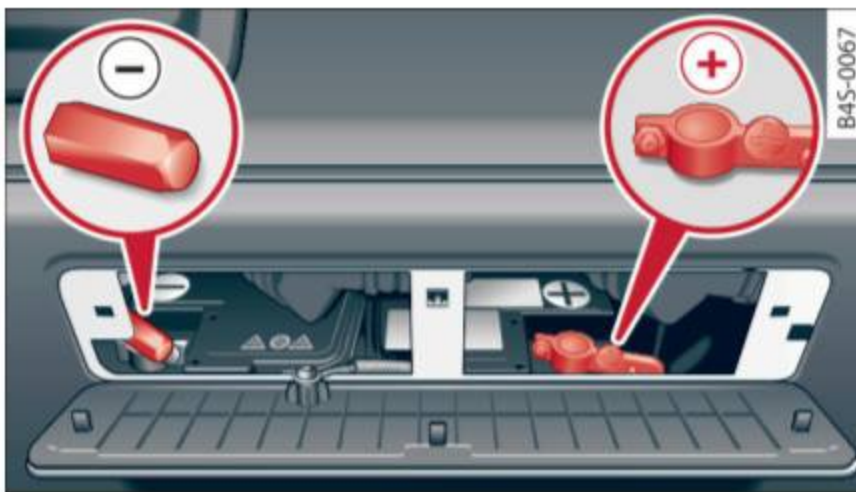
Fig. 186 Luggage compartment: connectors for jump start cables and charging unit
