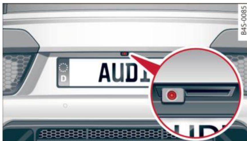
Fig. 75 Vehicle rear: rearview camera component location
