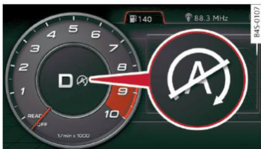
Fig. 59 Instrument cluster: engine stop temporarily unavailable
