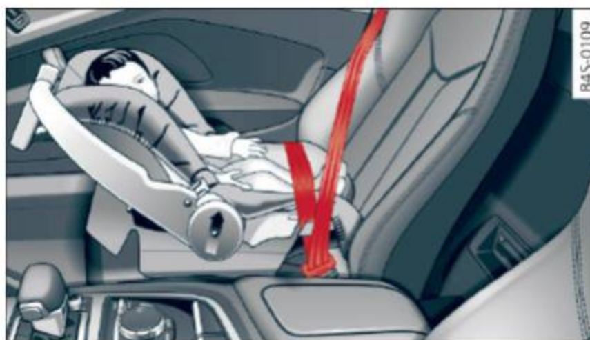
Fig. 154 Rearward-facing infant seat, properly installed on the passenger seat
