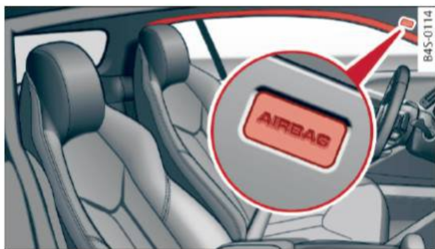
Fig. 152 Side curtain airbags, driver's side: side curtain airbag location
