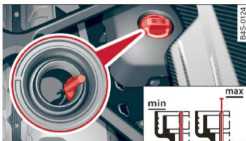
Fig. 165 Engine compartment: markings on the coolant expansion tank
