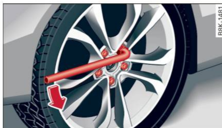
Fig. 179 Changing a tire: loosen the wheel bolts
