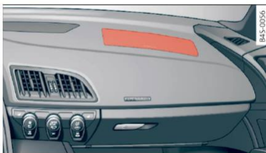
Fig. 145 Location of front passenger's airbag: in the instrument panel
