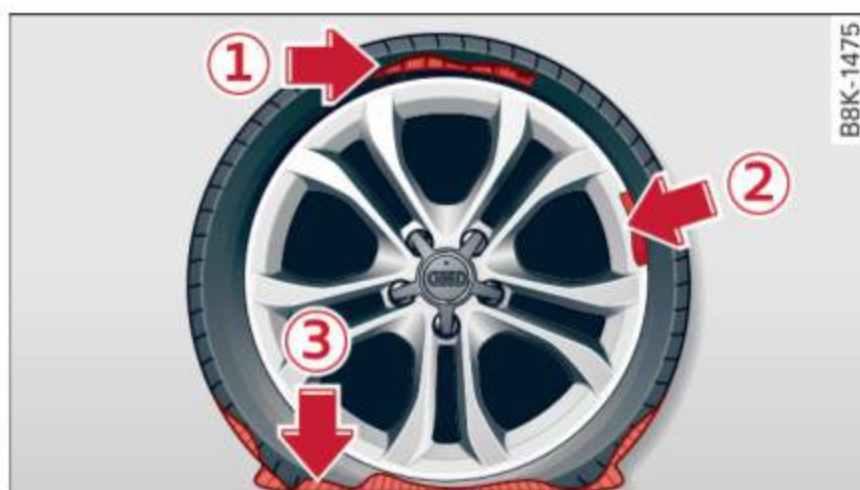
Fig. 175 Tire: tire damage that cannot be repaired
