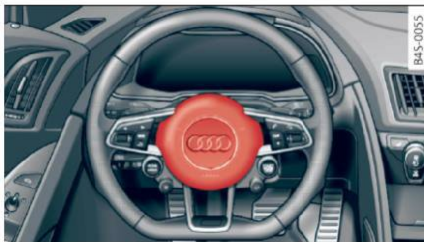
Fig. 144 Location of driver airbag: in steering wheel
