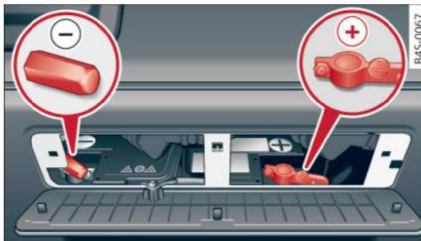
Fig. 167 Luggage compartment: connectors for a charger and jump start cables
