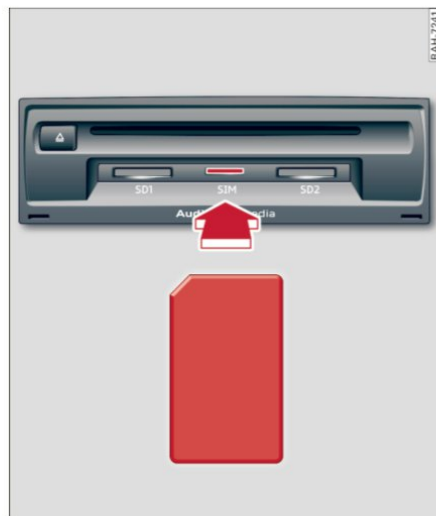
Fig. 104 Mini SIM card is pictured in actual size
