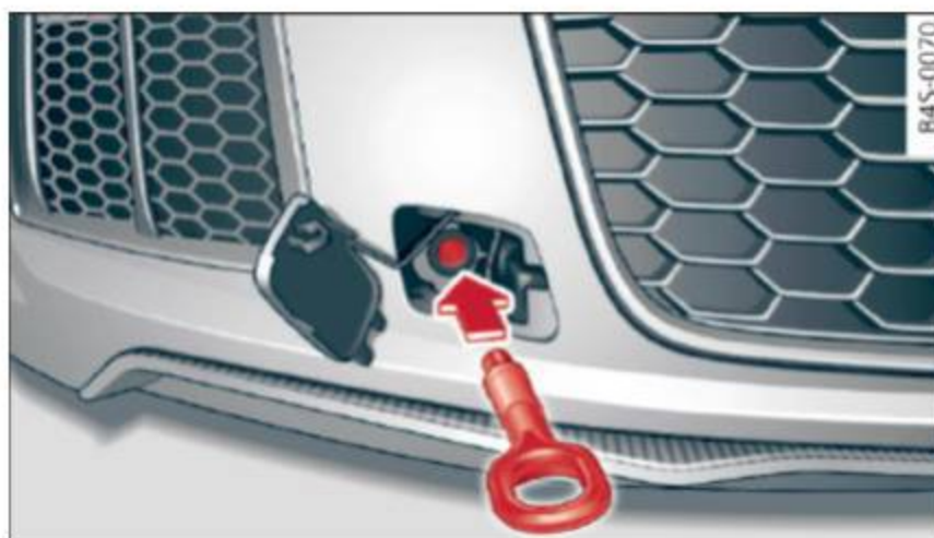
Fig. 189 Front bumper: installing the towing loop
