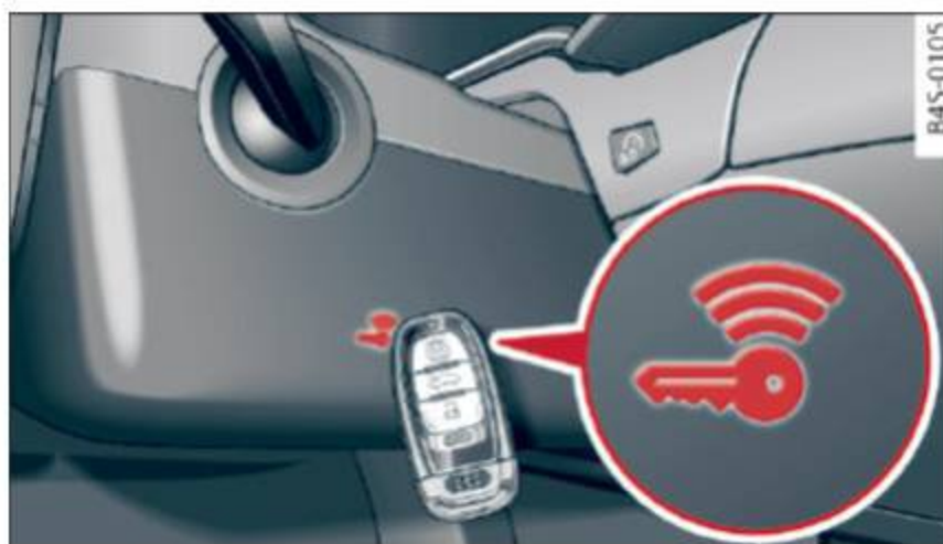
Fig. 57 Steering column/remote control key: starting the engine if there is a malfunction
