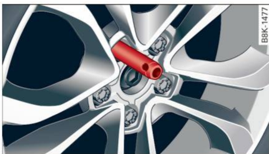
Fig. 183 Wheel: alignment pin in the top hole
