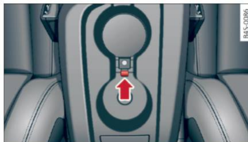
Fig. 65 Center console: parking lock emergency release cover
